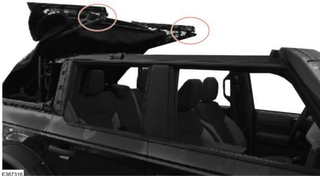
2. Inspect for the 6 circular hook and loop fasteners located on the soft top frame as shown in Figure 2. Do all 6 locations (3 on each side) have hook and loop fasteners installed and properly secured to the frame? (Figure 2)
