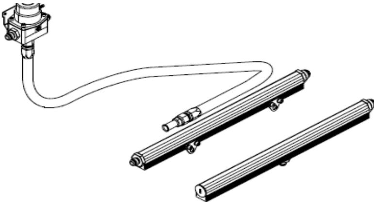
37. Connect one AN-06 straight hose end to each of the two ports on the fuel pressure regulator. Connect one AN-06 90-degree hose end to each of the AN-08/AN-06 reducer unions on the fuel rails. Plan a route for each of the two lines between the fuel pressure regulator and the fuel rails, measure the two lengths of fuel line needed. (See section titled Hose and Fitting Assembly) Once the hoses are assembled, **ensure there is no debris in the hose** and install them.
