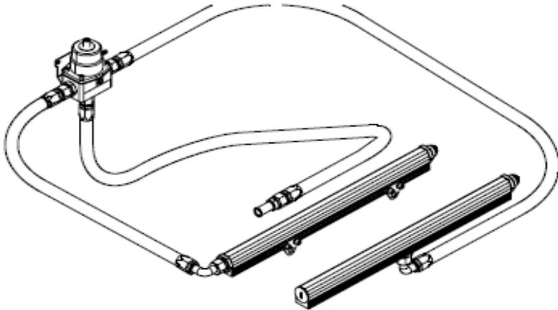
38. Inspect the OEM fuel supply line o-rings and replace if necessary. Place a light coat of oil on the fuel supply line o-rings and the supply line adapter fitting to ease installation. Connect the AN-08 tee adapter fitting to the OEM fuel supply line.
