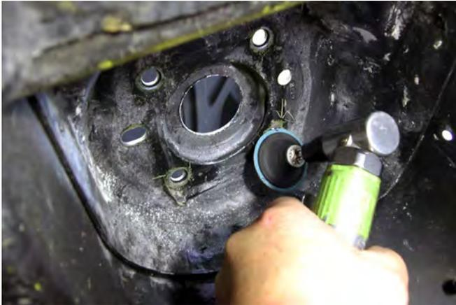
NOTE: Do not tighten the MM Caster/Camber Plate mounting nuts until instructed to do so. Thread the nuts on by hand until the tip of the bolts touch the Nylock portion of the nut.
