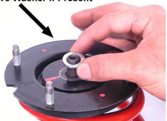
15. Remove the upper strut mount assembly from the strut shaft.
