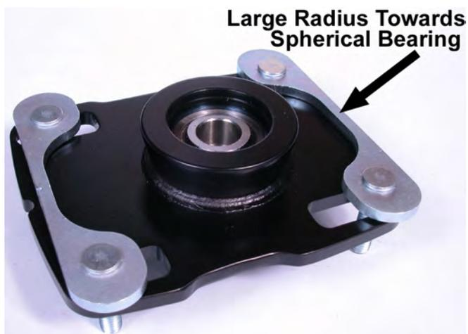
3. Place the passenger side Caster Plate on top of the passenger side Bearing Plate, making sure that the raised lip around the spherical bearing protrudes up through the center slot of the passenger side Caster Plate. The Caster Plate notch should be aligned with the Bearing Plate notch, and both are oriented towards the out-board side of the car.
