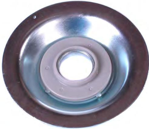
NOTE: The Bearing Plates are *not* side specific, but they must be correctly oriented during installation in order to properly function. For correct orientation, the circular notch on the Bearing Plate must face towards the outboard side of the vehicle and the spherical bearing must be below the Bearing Plate.
