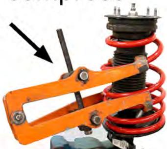
14. Remove the upper strut-retaining nut, and washer if present.
