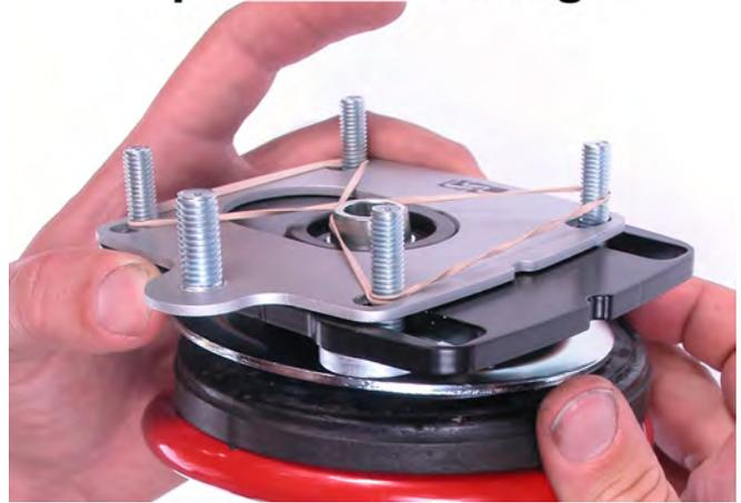
23. Reinstall the upper strut retaining nut, and washer if used, and torque to the manufacturer's recommended value. If using OEM or Tokico struts, torque to 45 lb-ft. If using Bilstein or H&R struts, torque to 54 lb-ft.
