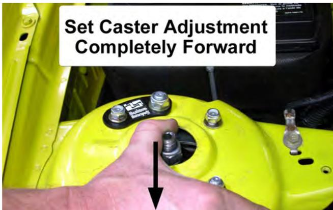
35. Next, center the strut shaft in the strut tower opening side to side. Once centered, torque the four 8mm Nylock nuts to 20 lb-ft.
