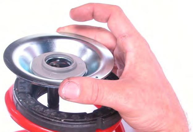
21. Place the spacer stack configuration shown below onto the strut shaft and into the spherical bearing. Ensure that the tapered spacers are properly seated against the shoulder of the spherical bearing.
