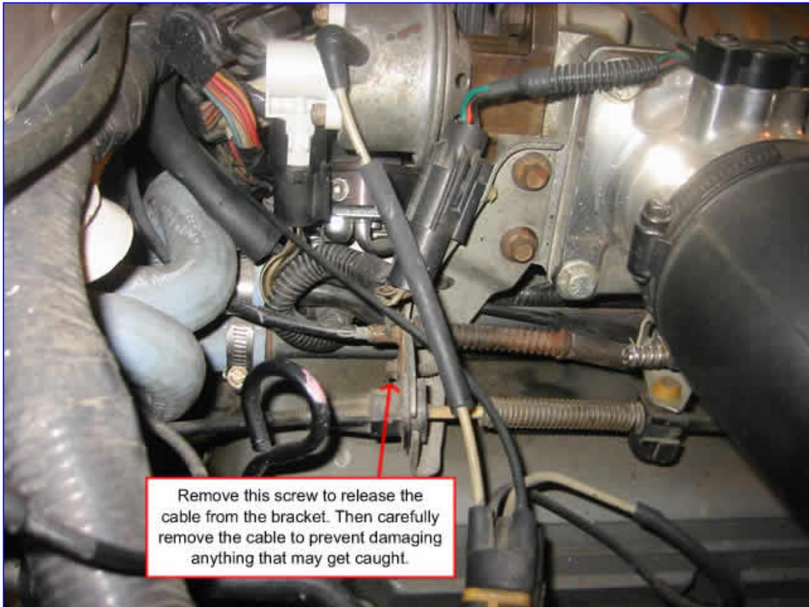
Remove this screw to release the cable from the bracket. Then carefully remove the cable to prevent damaging anything that may get caught.
