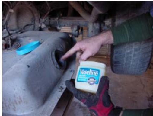
17. Put some petroleum jelly on the filler neck seal to help the filler neck slide into place.
