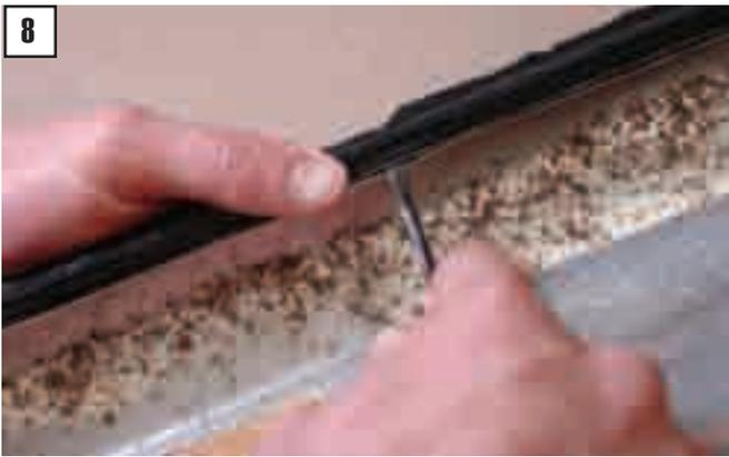
Now the destruction begins! Start by taking the flat blade screwdriver and loosening the staples that retain the inner door belt weatherstrip. Take the diagonal cutters and remove all of the staples and lay the weatherstrip aside for reuse later. Or if you are replacing the weatherstrip, just chunk it.
