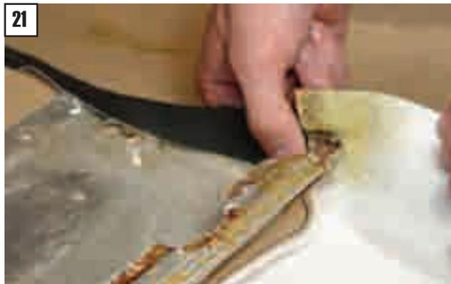
Now that you have the vinyl all ready to be glued, take the spray adhesive (after it is properly shaken) and apply glue to the back corner (the corner that will be toward the rear of the car when the panel is installed). Once positioned hold the vinyl tightly in place for a minimum of three minutes. Move to the front corner and repeat the last step
