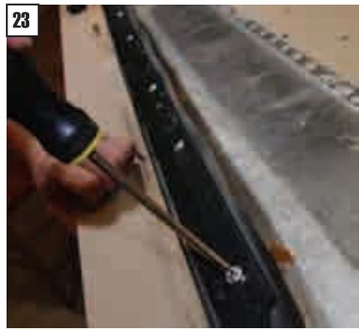
To finish up, grab your extra set of hands and your inner door belt weatherstrip and screws. Pull the remaining unglued vinyl and pull it tight. Position the inner door belt weatherstrip and install a screw in the center, then put a screw in each end. You will use six screws per panel.
