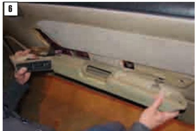
Now lift up and pull out on the armrest, but be careful because the power window switch wiring will still be attached to the armrest. Depending on year model, you will either have two plugs for your window switch wiring, or you will need to take your phillips head screwdriver and remove the two screws retaining the switch plate to the switch cover.
