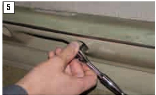
Take the flathead screwdriver or a pocket knife (finally a different tool!) and remove the two armrest hole plugs. Use the 10mm nut driver or ratchet setup to remove the two screws retaining the armrest.
