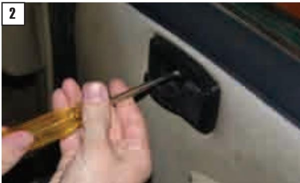
Then use the phillips head screwdriver to remove the door handle bezel.
