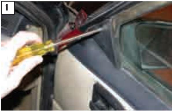
Start off by removing the mirror hole cover with the phillips head screwdriver.
