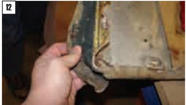
With the grommet removed, peel the vinyl off of the metal door panel piece.
