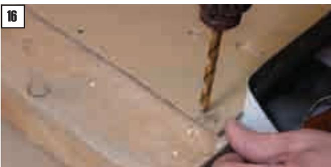
Following all applicable safety precautions for electric drill usage, drill the holes in the board. Then run the drill through the corresponding holes on the metal to ensure that the rivet will pass freely through.
