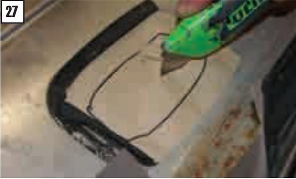
Lay the panel face down cut out the areas for the armrest. For the door handle, grab your old vinyl and lay it over the new panel. Trace the hole and cut it out. Some trimming may still be required after the panel is installed.
