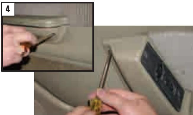
Then remove the two screws (one located at each end) from the armrest, still using the phillips head screwdriver.
