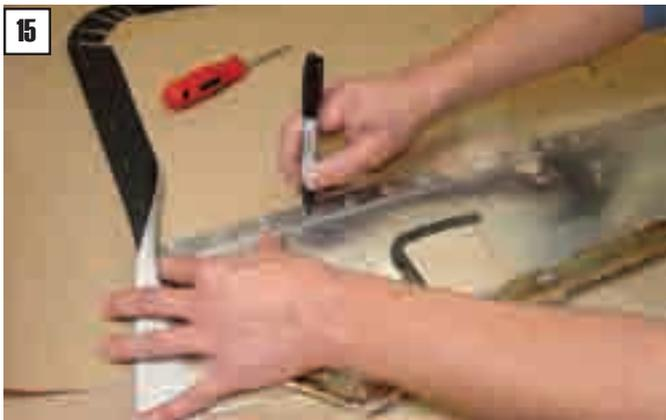
You will notice that the metal upper door panel has a "lip" at the lower edge. You will need to position the new board on the upper part (the side that will face toward the cars interior), center it, and mark your holes to be drilled. (Here is where the extra set of hands may be needed.) *\*Removal of the upper most staples retaining the vinyl to the board may be necessary to obtain proper access to the board*
