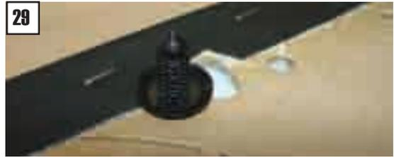
Install your new door panel clips. This is simply done by sliding the clip head first into the large opening of each retainer slot and pushing it towards the smaller opening until it "locks" in place.
