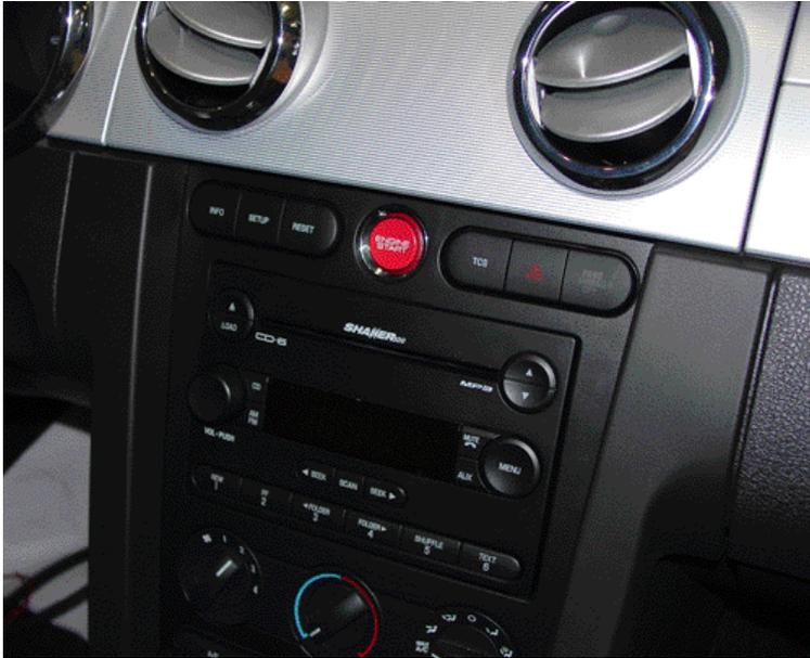
We hope you will enjoy your new custom push button start ignition. Please make sure that the button is not pushed more than once when starting the vehicle, or once the vehicle is running. This could cause a short in the circuitry.
