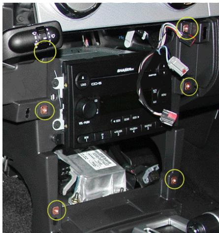
Use a 7mm socket to remove the 6 small retaining bolts which hold the radio/AC bezel in place. Slowly pull the bezel forward and disconnect the 3 switch harnesses at the top. Pull it slightly more forward and disconnect the HVAC switch harness on the bottom right. Be careful with this connector. It is a lever-style connector which must have the small clip pushed in and then the lever pulled forward for removal.
