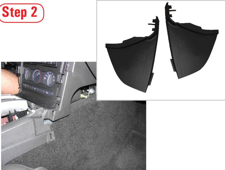
Next, pop the 2 center console side panels off by simply pulling up and back towards the rear of the car.
