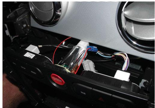
Now, you can re-attach all other connections on the back of the radio bezel including the HVAC connection.
