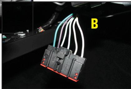
Now we are ready to re-wire the ignition. Located on the left side of the steering wheel column you will find the ignition wiring harness (A) plugged into the side of the column. Unplug the harness from the steering column to where it hangs freely (B).
