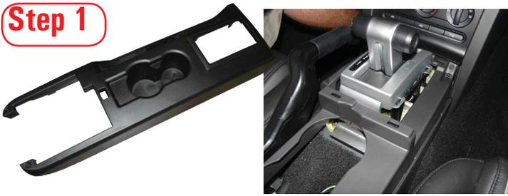
First, the top center console housing will need to be removed. This is done by simply opening the center console compartment and removing the 2 connecting screws at the base of the lid. Pull the emergency brake lever up and pop the rest of the housing off and slide it over the emergency brake lever and shifter.
