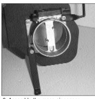
8. Assemble the mass air sensor, adapter, gaskets and brackets using the hardware provided.
