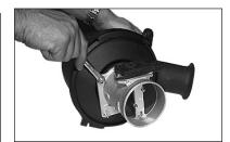
6. Loosen and remove the four nuts that retain the mass-air sensor to the air cleaner.
