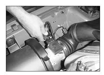
2. Disconnect the mass air sensor electrical connections.
