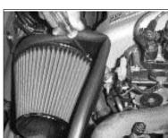
15. Install the filtercharger element onto the adapter and secure it with the hose clamp provided.
