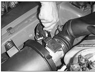
3. Loosen the hose clamp on the intake tube at the mass air sensor.
