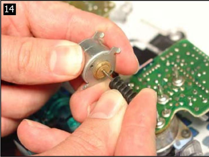
15. Be sure to not push the gear on too far, leave a small air gap between the motor & the gear.
