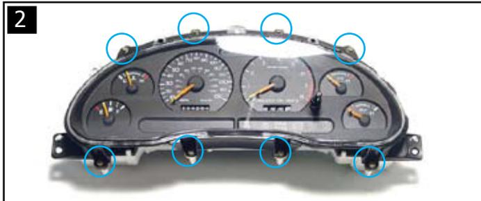
2. Remove the 8 T15 torx screws that hold on the instrument cluster lens.
