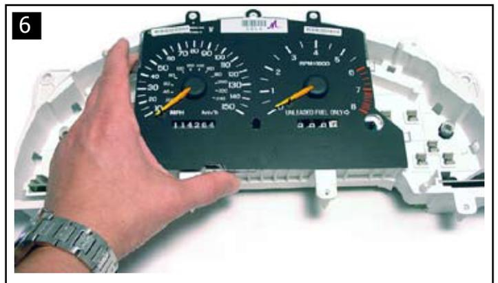
7. Flip the speedometer/tachometer over so that the back is facing upward.
