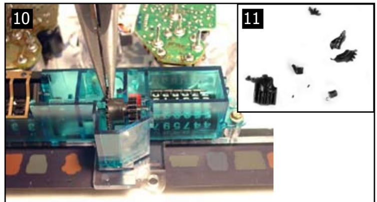
12. Install the new drive gear by pushing it down until it snaps in to place.
