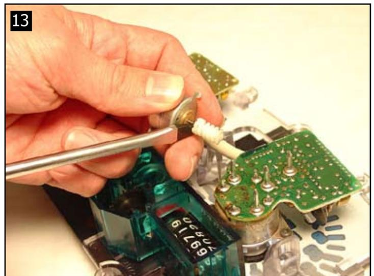
14. Install the new drive gear by simply pushing it on.
