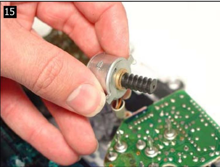
16. Re-install the odometer drive motor by pushing down & turning counter clockwise at the same time.
