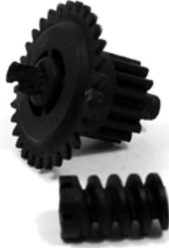
**So your odometer quit working, but your speedometer still registers the correct speed. The most likely cause is not the speedometer itself, but the plastic gears used to drive the odometer. Follow these simple instructions to get your odometer back on track.**
