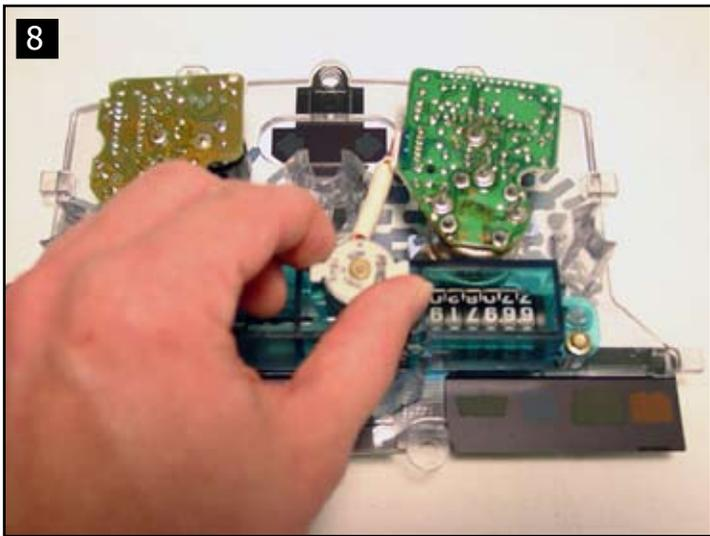
9. With the odometer drive motor released, you can see the drive gear attached to the motor & the black driven gear still in the gauge.
