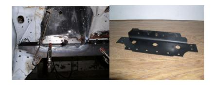
The bottom plate with the three large holes is to weld the crush tubes onto. Check the plate in the rail to be sure the holes line up for the k-member support bolts and now that you know what side goes up you can tack weld the crush
