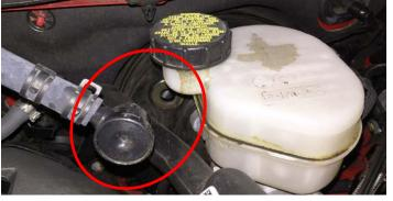
39. Remove the sound generator assembly and plug the hole in the firewall using the supplied plastic grommet plug supplied in Bag # 1.
