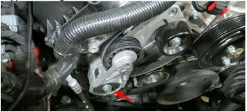
60. Using the M8 x 20mm bolts and M8 washers supplied in Bag # 2, install two idler pulleys to the tensioner bracket. The top idler pulley is 65mm and the lower idler is 76mm. Add a small amount of blue thread lock fluid to the threads ONLY, do not allow excess thread lock fluid to drip onto the pulley's bearings. Torque the bolts to 18 ft-lbs.
