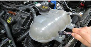
86. Install the supplied coolant bleed hose and secure with the factory hose clamps.
