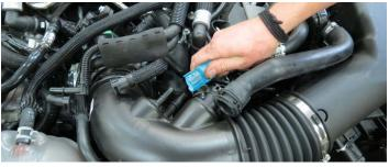
33. Remove the additional brake aspirator hose from the air inlet tube.
