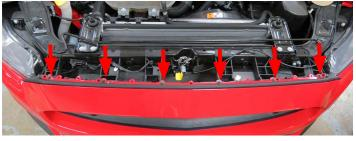
20. Using a 5.5mm socket, remove two (2) bolts under the weather stripping, one per side.
