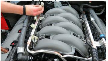
45. Place a rag underneath the fuel input line. Lift up the blue locking tab and disconnect the fuel line from the rail.
