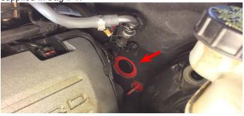
40. Remove the passenger side PCV hose from the valve cover and the intake manifold.
