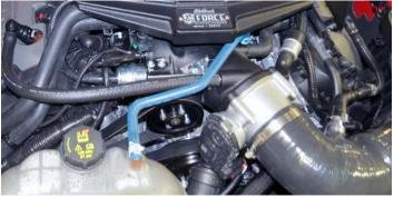
87. Carefully remove the protective foam from the brake aspirator.
