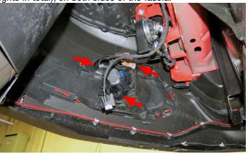
26. Tape up the fender as needed to prevent scratching the painted surfaces. With the help from an assistant, carefully disengage both sides of the fascia by gently pulling the sides outwards. Remove the fascia and set aside.
