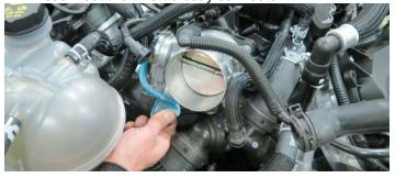
42. Using an 10mm socket, remove four (4) bolts securing the heater hose retaining brackets.
