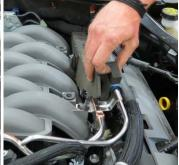
44. Disconnect eight (8) fuel injector connectors.
