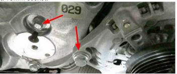
57. Secure the idler bracket by installing bolts from Bag # 2. The M10 x 110mm bolt through the ear of the alternator, the M8 x 90mm bolt into the top front cover hole, and the M10 x 45mm bolt through the lower hole that was used to secure the stock tensioner. Use blue thread lock fluid on all of the bolt threads and torque all bolts to 22 ft-lbs.
