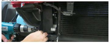
97. Using a drill and a 1 1/4" hole saw bit, drill a hole in the shroud that lines up vertically and parallel with the upper LTR barb. *CAUTION*: Be mindful of the A/C hard lines behind the shroud.
