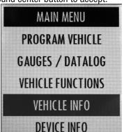
Follow the on-screen instructions. When prompted to do so, turn the vehicle's ignition ON but do not start the engine. Press the round center button to accept. The ECU Strategy and SWPN will be displayed on the following screen.
