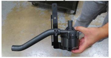
99. Feed the hose through the hole in the shroud and secure the water pump to the chassis using the supplied nuts in Bag # 3.
