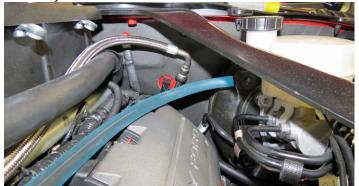
91. Route the Aspirator to Manifold hose under the heater hose and attach to the fitting on the supercharger nose.
