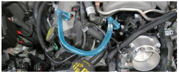
41. Disconnect the throttle body connector.
