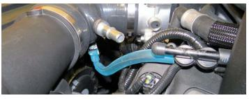
120. Connect the 90° fitting on the supplied driver side PCV hose to the driver side valve cover. Connect the other end to the fitting on the silicone elbow.
