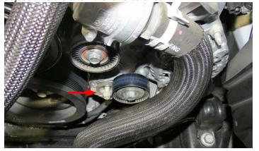
56. Remove both the engine cover bolt using a 10mm socket and the bolt through the ear of the alternator using a 15mm socket.
