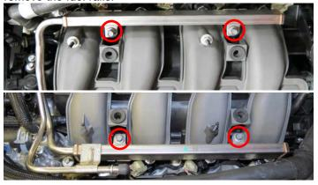
47. Using an 8mm socket, remove six (6) manifold bolts.
