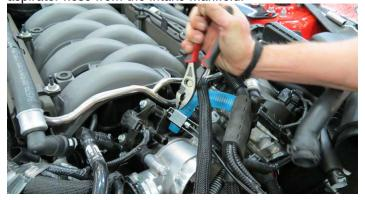
38. Remove the brake aspirator hose assembly from the brake booster and set aside as it will be reused later.
