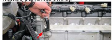
65. Using a hose clamp tool, remove the factory coolant bleed hose from the reservoir and bleeder fitting.
