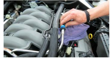
46. Using a 10mm socket, remove four (4) bolts securing the fuel rail and manifold. *TIP:* It's not required to fully remove the fuel rails.
