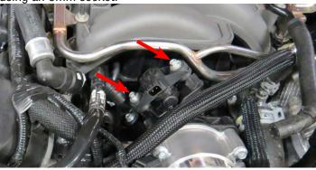
70. Install the EVAP solenoid to the supercharger manifold using two (2) M6 x 25mm bolts in Bag # 1.
