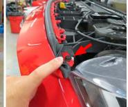
21. Remove sixteen (16) bolts and six (6) push pins securing the splash guard using a 7mm socket and a panel puller. Remove the splash guard and set aside.
