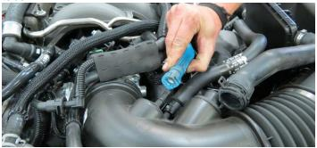
32. Remove the driver side PCV hose from the air inlet tube.
