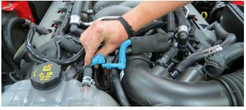
35. Using a flathead screwdriver, loosen two (2) worm clamps securing the air inlet tube and remove.
