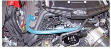
108. Using a razor blade, remove the 90° fitting on the factory EVAP hose.
