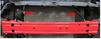
93. Secure the LTR brackets to <u>both</u> sides of the LTR using the M6 x 10mm bolts from Bag # 3.
