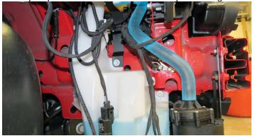
104. Secure the Surge Tank to Manifold hose to the surge tank and manifold using two (2) hose clamps from Bag # 3.
