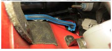
37. Using a hose clamp tool and pliers, remove the brake aspirator hose from the intake manifold.
