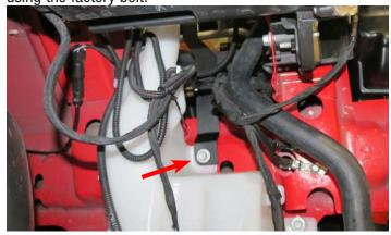
106. Using a razor blade, or equivalent, remove the 90° quick connect fitting on the factory passenger side PCV hose.
