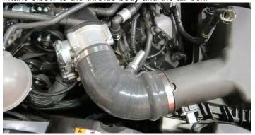
119. Connect the brake aspirator to the lower fitting on the silicone elbow.
