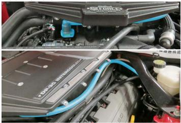
110. Connect the supplied straight quick connect fitting on the EVAP hose to the hard line.
