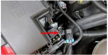
112. Open the fuse box and using a 10mm socket, attach the "Power Supply Wire" on the Water Pump/EVAP Harness to the power terminal on the fuse box.
