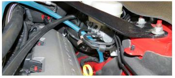
111. Zip tie the Fuse holder on the Water Pump/EVAP Harness onto the top right corner of the fuse box.
