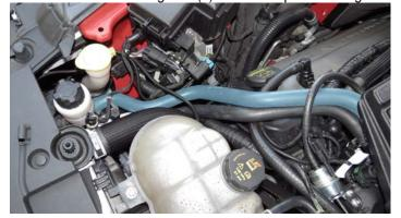
105. Using a 10mm socket, remove the top bolt securing the windshield wiper fluid reservoir. Place the surge tank bracket onto reservoir and secure the bracket and reservoir using the factory bolt.
