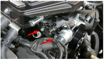
71. Using O-ring lube, install the fuel rail fittings onto the fuel rails. The passenger side rail will have the black plug on the front of the rail, while the driver will have the 180° fitting. Attach the supplied fuel crossover to the rear of both rails.
