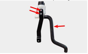
103. Connect the Water pump to Surge tank hose to the water pump and secure with a hose clamp from Bag #3.
