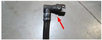
107. Attach the 90° fitting onto the supplied 1/2" Cadbar hose. Connect the quick connect fitting to the passenger side valve cover and the other end of the hose to the barb on the supercharger nose.
