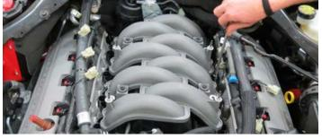
48. With the manifold bolts removed, carefully position the manifold forward and remove four (4) sensor connectors and two (2) harness clips.
