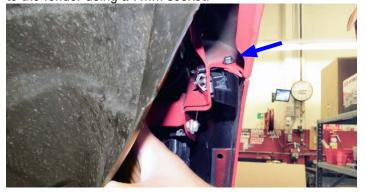
25. Unplug the fog lamp and signal light connectors (3 lights in total), on both sides of the fascia.
