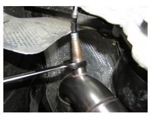
With all of the sensors installed and tightened, connect the sensor connectors into the appropriate extension cable
