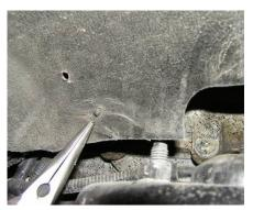
Remove the front skid plate if installed to expose the underside of the engine bay. Normally this not included with the 2WD model.
