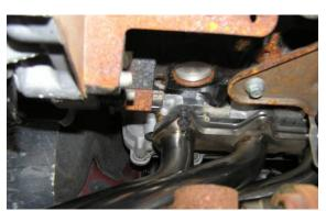
Note: The "keeper clip" on the round portion of the cable extension where it plugs into the mating part in the wiring harness serves to locate/index the wiring to the O2 sensor. The small tabs placed around the outside of the connector barrel may or may not need to be ground or cut off. The OEM manufacturer may use a slightly different connector as far as these additional keys are concerned but have no bearing on how the connectors go together because of the "keeper clip".
