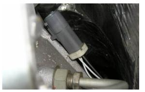
Note: 02 sensors are delicate electronic components and should be handled very carefully. Take extra care in not contaminating the sensing end with shop towel lint, finger prints, oil, etc.
