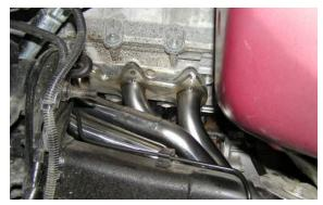
• Install all of the prepared bolts in the left (driver) side. Be sure to screw them in by hand several turns to guard against cross-threading.
