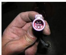
Notice the connectors with the external tabs removed to allow for plug in.
