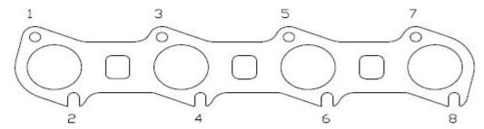
USE THIS CHART TO TORQUE THE HEADER BOLTS ON BOTH THE LEFT AND RIGHT FLANGES. TORQUE EACH BOLT TO APPROXIMATELY 20 FT/LBS.
