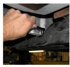
• Next move to the left (driver) side to install the oil dipstick tube. Place a small amount of motor oil on the O-ring at the end of the tube and slip the end of the tube into the block.
