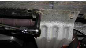
Next, loosen the nuts on the clamp between the stock
