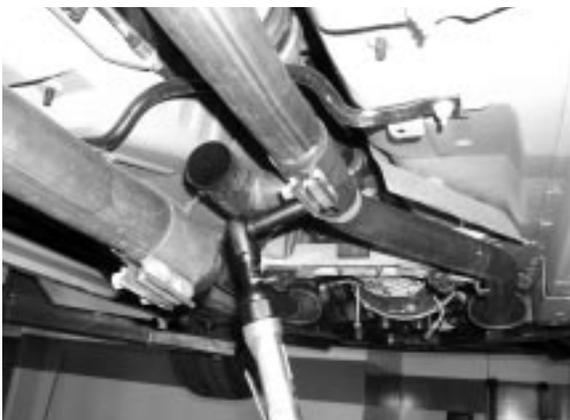
Separate H-pipe from tail pipe.
