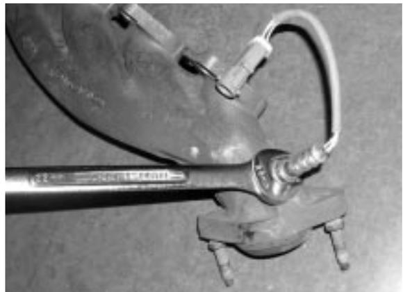
Removing the oxygen sensor.
