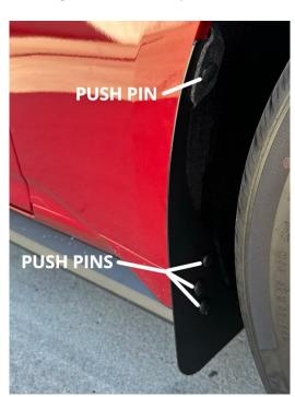
Once the front push pins are removed you can now place the rock guard up to the vehicle and you will want to slide the guard behind the inner fender liner up top and place the push pin back in. Now align the lower holes to the push pin holes and place those back into the car and the front guards are now installed.
