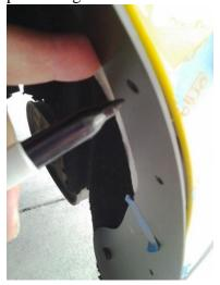
8. The blocks must be pre-drilled for the included self-tapping screws. Use 1/8" (min) to 5/32" (max) drill bit.
