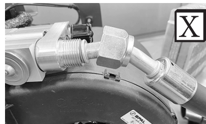
Improperly Seated O-ring Land
