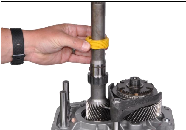
8.23: Install mechanical speedometer gear with detent ball to main shaft (Note: Ford=12 tooth; GM=17 tooth)
