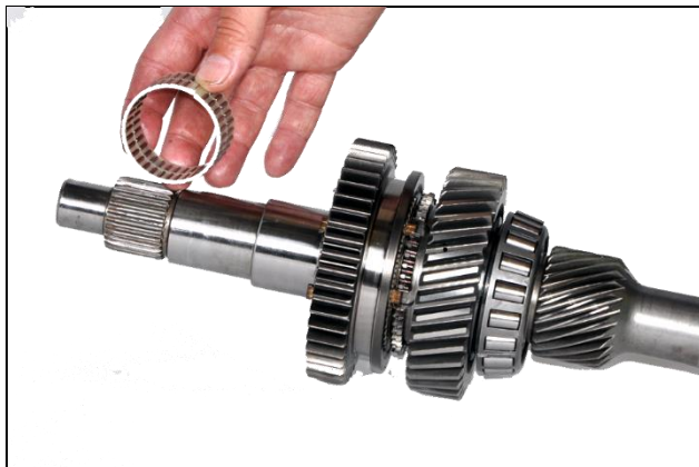
6.11: Install 2 nd gear bearing onto main shaft
