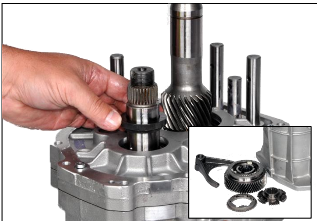
3.27: Remove 5 th gear thrust washer 3.28: Remove steel locking ball under thrust washer
