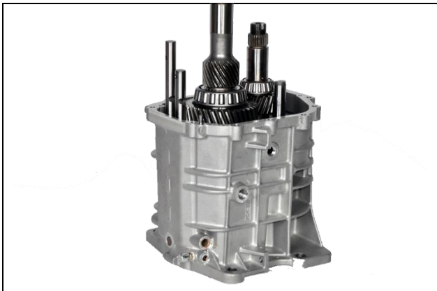
8.3: Install main shaft and fork assembly into main case. Use a 2 1/2" (round) x 1" (thick) spacer on the table to hold main shaft.
