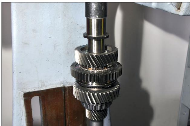
6.13: Press 3 rd gear thrust washer and bearing journal onto main shaft
