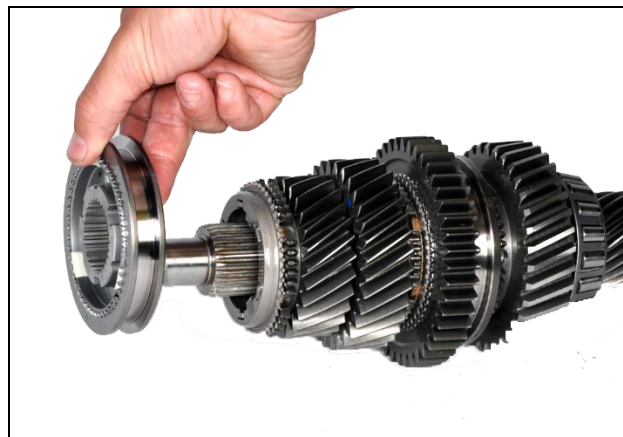
6.16: Install 3 rd gear blocking ring 6.17: Press 3-4 synchronizer onto main shaft. Be careful to align blockers into tabs on synchronizer
