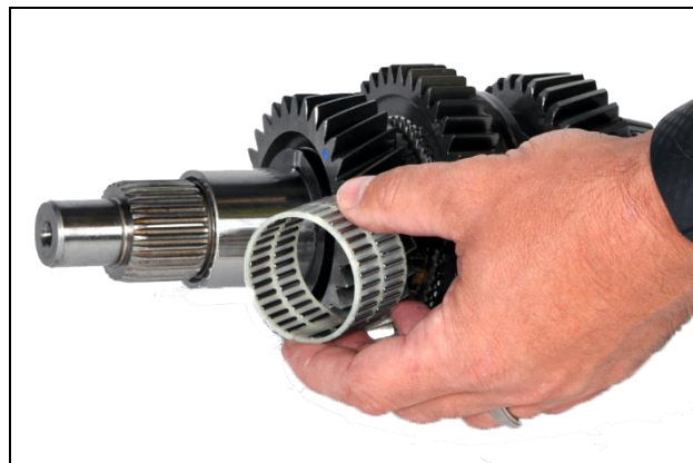
6.14: Install 3 rd gear roller bearing and bearing thrust sleeve onto main shaft
