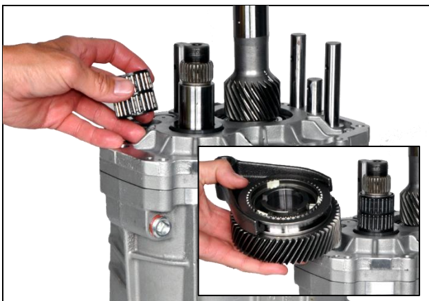
8.18: Install 5 th gear bearing to cluster shaft
