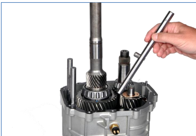
3.34: Rotate 5 th reverse shift rail counter clockwise and remove from case
