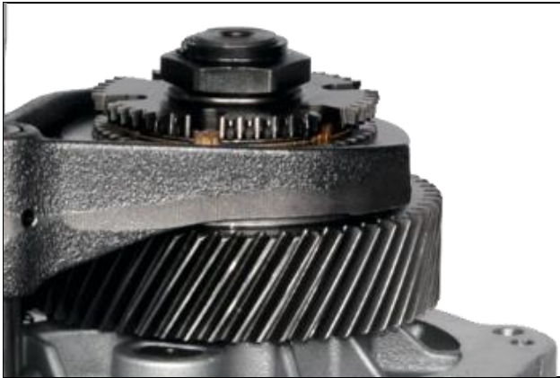
8.21: Install counter shaft locking nut
