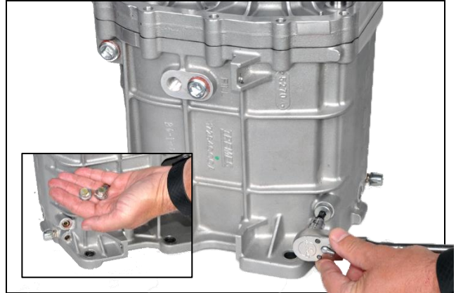
3.38: Remove two shift rail detent plugs
