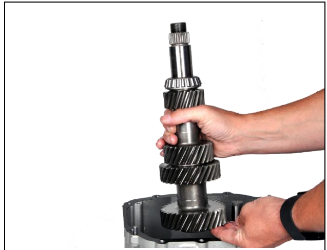
3.42: Remove cluster shaft from case
