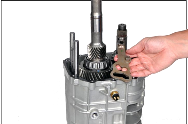
3.37: Remove shift selector link from case
