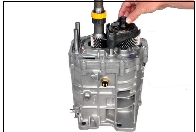
3.16: Position transmission in vertical position to access rear
