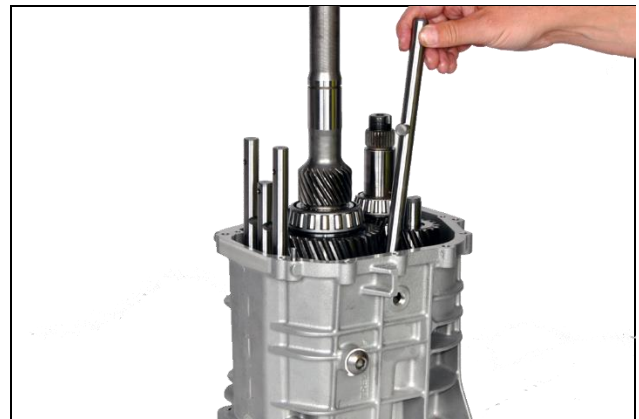
8.10: Install 5 th reverse shift rail into case (Note: Rail detent roller fits in selector arm)
