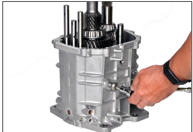
8.6: Install pivot pin into selector on side of main case. Torque to 25-40 lb-ft
