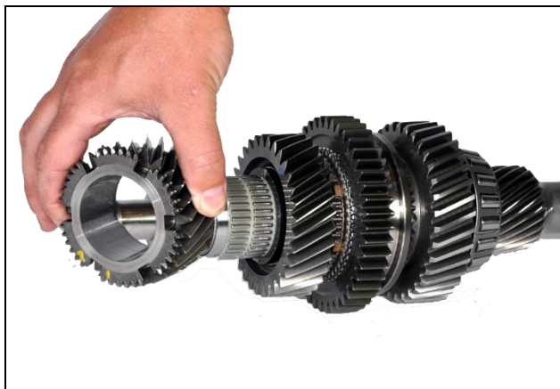
6.15: Install 3 rd gear onto main shaft
