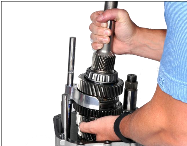
3.40: Remove main shaft assembly with 1-2 and 3-4 shift fork and rail assembly
