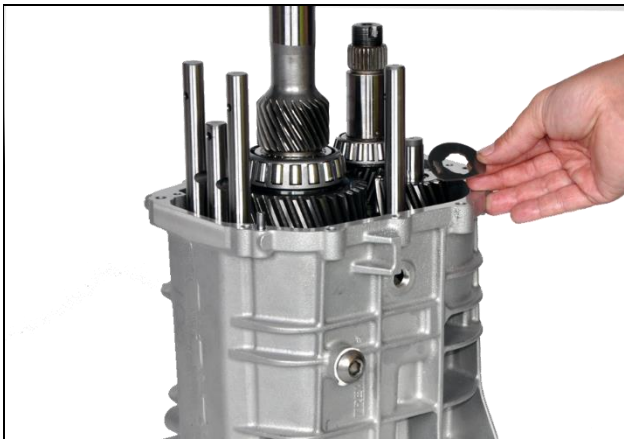
8.11: Install reverse gear thrust washer on top of idler gear (Note: Place tab in the 12 o'clock position)
