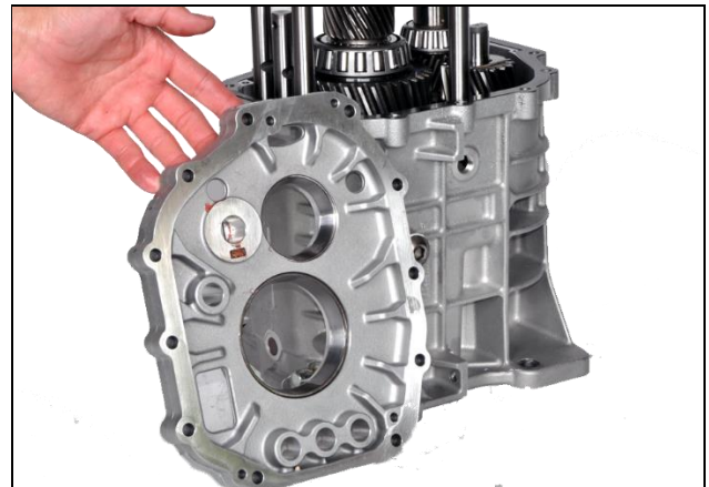
8.12: Install rear housing gasket and intermediate plate. (Note: Be careful to line up idler gear thrust washer.)
