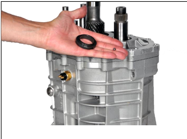
8.16: Install 5 th gear bearing and thrust washer to cluster shaft
