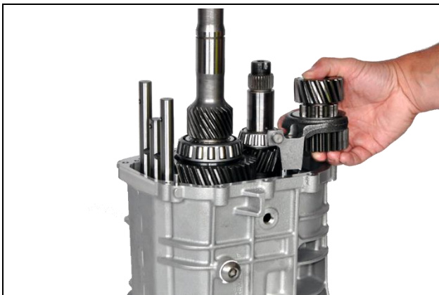
8.9: Install reverse idler synchronizer and fork into case
