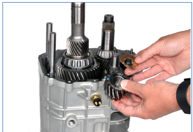
3.35: Remove reverse idler gears and synchronizer from case
