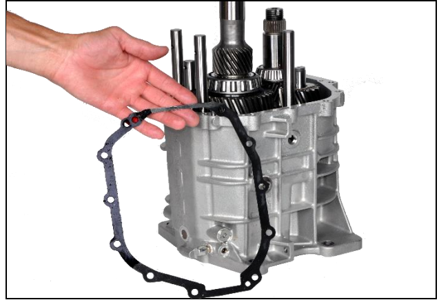
3.31: Remove extension housing gasket
