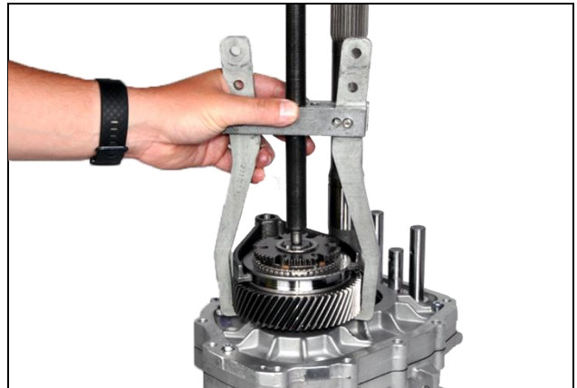
3.26: Using a two-jaw puller, remove 5 th gear and synchronizer assembly
