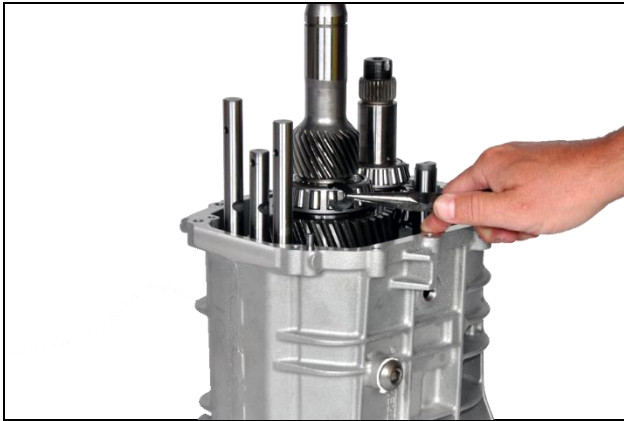
8.7: Install pivot pin snap ring
