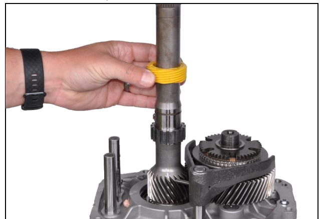
3.19: Remove mechanical speedometer gear
