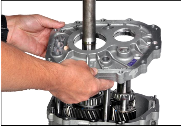
3.30: Remove mid-plate from main case
