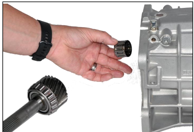
8.28: Install input shaft and pocket bearing
