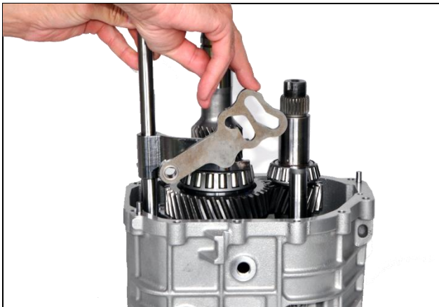
8.5: Install 5 th and reverse gear selection arm into case
