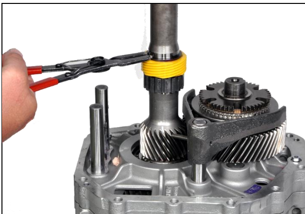
3.18: Remove speedometer gear snap ring
