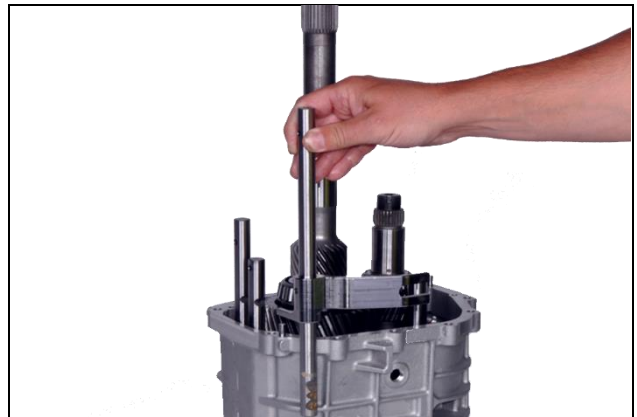
8.4: Install 5 th and reverse gear fork and rail into main case
