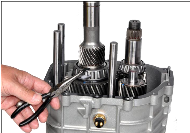
3.32: Remove snap ring from 5 th reverse selector link inside main case
