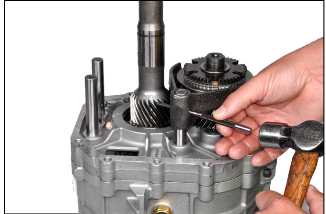
3.23: Remove 5 th gear fork roll pin
