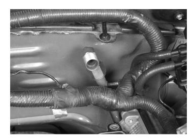
4. Bend steel tab down on wiring harness bracket.
