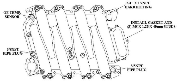
1. Install supplied 3/4" barb fitting and pipe plugs into lower manifold. Use a small amount of liquid Teflon sealer on threads. Install Upper to lower gasket first then install studs.
