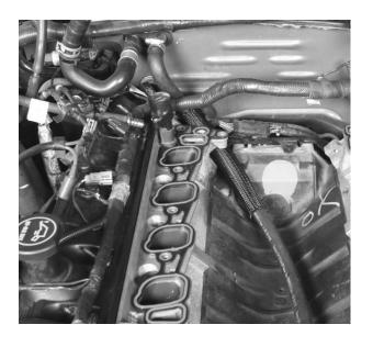
3. Bend EGR tube toward driver side of vehicle so that the vertical portion of the tube is aligned with top end bolt boss on cylinder head. Cut EGR tube with tubing cutter 4.25" above intake face and install 90 degree compression fitting. Do not fully tighten compression nut, this will be done later in the installation.
