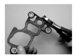
5. Install new intake gaskets. Some gaskets have tabs located on the passenger side rear that will need to be trimmed off for clearance.
