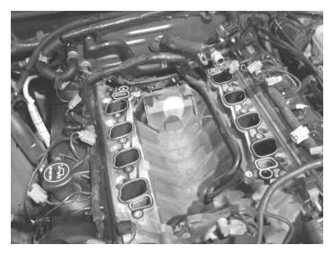
OE PI Upper and lower Manifold Removed from Vehicle.
