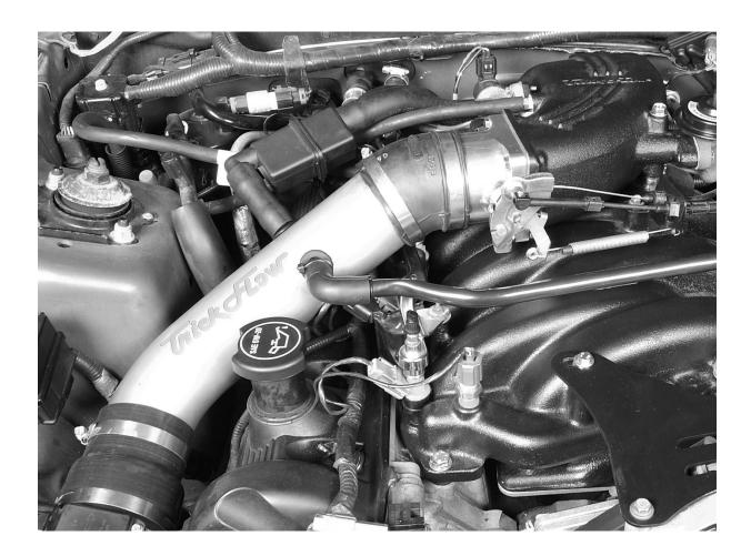
14.Install throttle/cruise cables and bracket. Cable bracket mounts upside down from OE. Modify bracket by drilling out the round hole to 3/8" dia., this will allow some adjustment for different manufactures throttle bodies and OE Ford factory tolerances.
