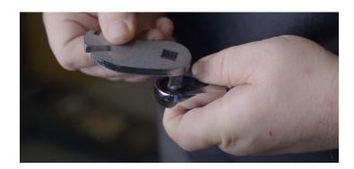
Before using the SVE pinch weld jack pads, please verify that the pinch weld area is straight. If it isn't, use the flange tool to straighten the pinch weld near the factory recommended jacking points. (Please note: Some pinch welds may need to be repaired by a trustworthy, professional body shop.)
