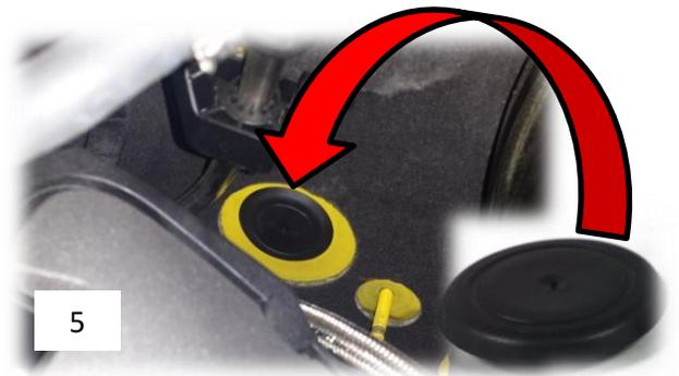
Figure 5: Sound tube plug installed
