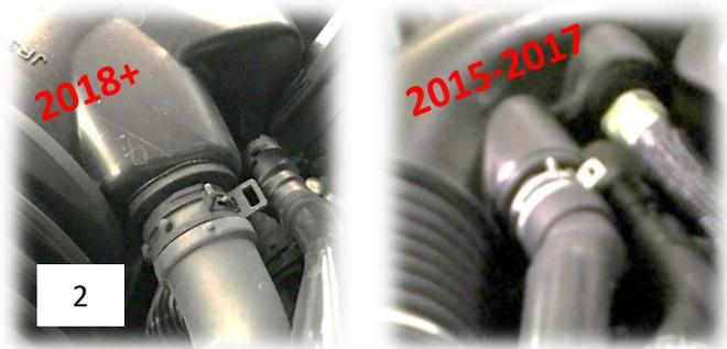
Figure 2: Hoses connected to factory intake tube
