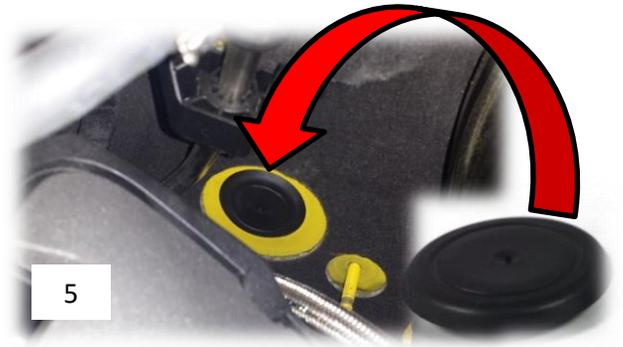
Figure 5: Sound tube plug installed
