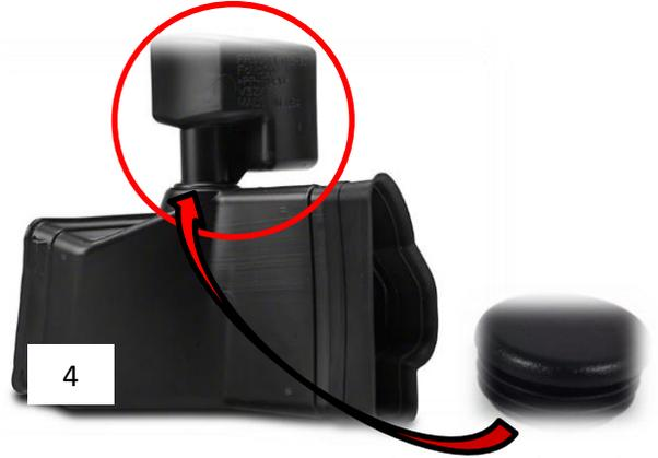
Figure 4: Factory resonator on inlet duct and Steeda plug
