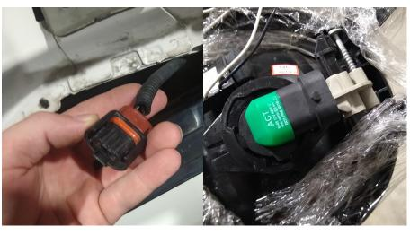
**Step 2:** Attach factory fog light connectors to the fog light bulb.
