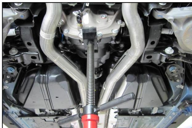
**32.** Support the differential using a jack as shown.
