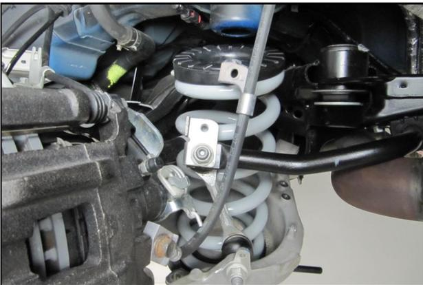
**37.** Transfer the OEM isolator onto the RTR Spring. Rotate the isolator in the spring until the coil end bottoms against the isolator
