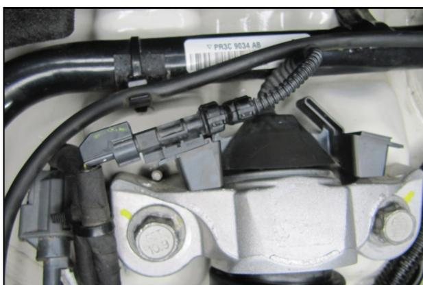
**46.** Reconnect the MagneRide harness at the top of the shock. Repeat steps 40-46 on the opposite side of the vehicle.
