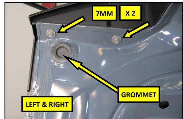
33. Secure the edges of Spoiler using the OEM screws and reinstall the blind grommets removed in step 7.
