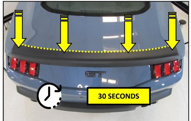
**37.** Press firmly onto the leading edge for a minimum of 30 seconds to achieve a strong bond.
