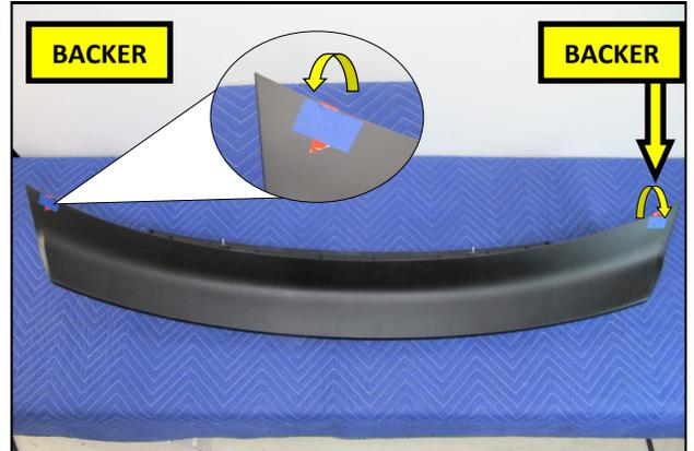
29. Tape the ends of the tape backer onto the top side of the RTR Spoiler as shown.
