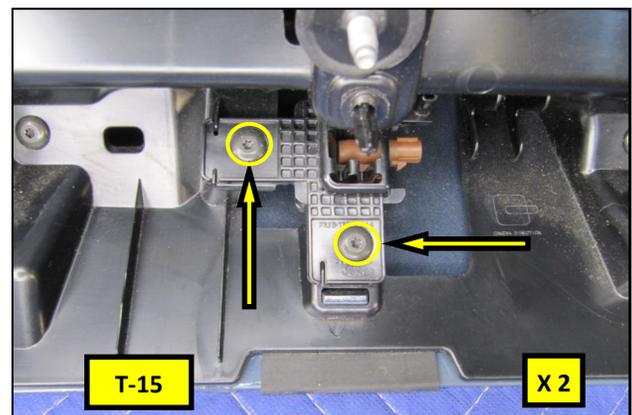
15. Place the decklid, face down, onto a padded work surface. Using a T-15 Torx driver, remove the two screws in the camera bracket.
