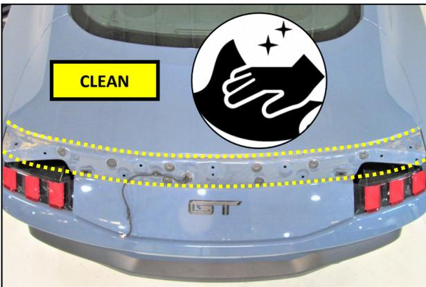
24. Using a mild solution of soapy water and a microfiber towel, remove any and all dirt that may have accumulated underneath the decklid.
