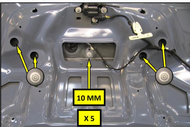
32. Secure the Spoiler using the OEM flange nuts removed in step 8. **NOTE:** Special care should be taken to avoid dropping the nuts into the trunk lid.
