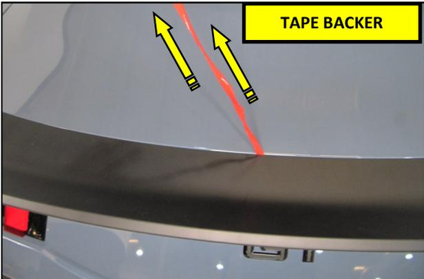
**36.** Carefully pull the tape backer out from underneath the Spoiler.
