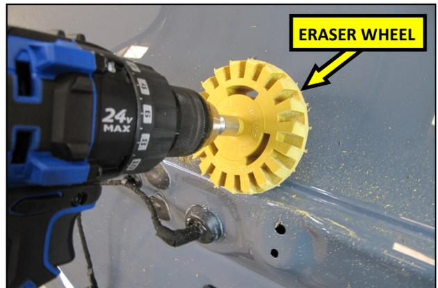
25. Using a rubber eraser wheel and a drill, remove any remaining adhesive on the trunk lid.
