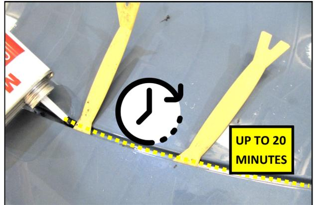
**NOTE:** depending on the age of the adhesive on the vehicle, this may require considerable effort to remove. Allowing the solvent to act for as long as 20 minutes will ease this process. Multiple applications may be necessary.
