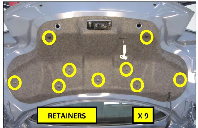
**4.** Using a panel trim removal tool, pry the 9 retainers from the liner.
