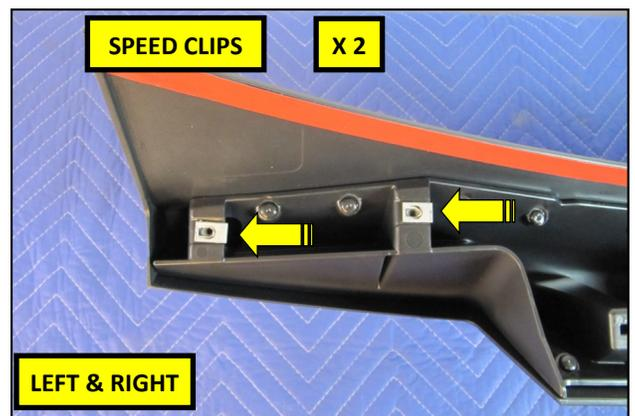
21. Reinstall the OEM speed clips from step 18 onto both ends of the RTR Spoiler.
