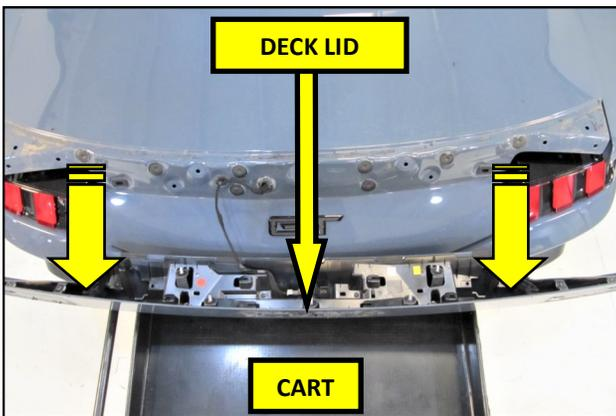
12. Remove the deck lid from the vehicle and set it onto a tool cart or similar.
