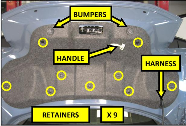
**34.** Pull the trunk release handle through the liner and install the bumpers to hold it in position. Reinstall the nine retainers into the trunk lid and pull the wire harness through the cut in the liner.
