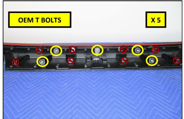
19. Transfer the T bolts from step into 17 into the RTR Spoiler.
