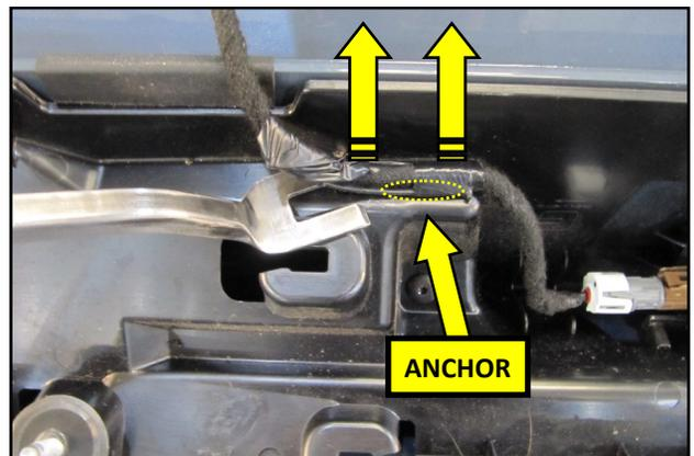
13. Using a panel clip removal tool, pry the harness anchor out of the deck lid.
