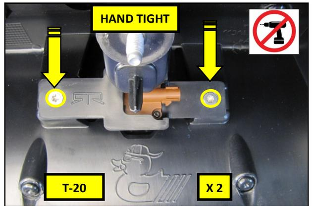
23. Place the camera and Bracket into the center of the RTR Spoiler as shown. Using a T-20 Torx driver and the supplied M4 Screws, secure the camera and bracket to the spoiler. Tighten the screws by hand to avoid
