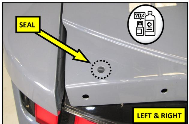
27. Using isopropyl alcohol, thoroughly clean the trunk lid surrounding the spoiler bolt holes. Carefully apply the Sealing Discs over the bolt holes as shown.
