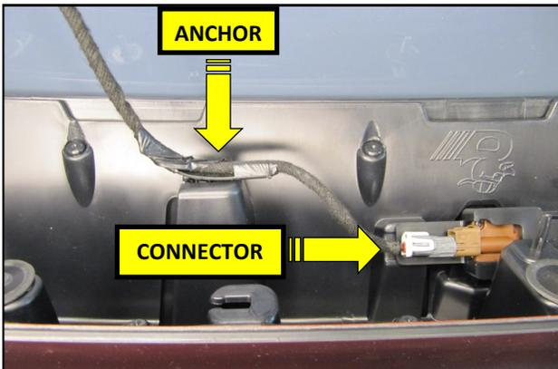
30. Place the RTR Spoiler onto a padded tool cart near the vehicle. Reconnect the camera harness and insert the anchor into the open T bolt slot, as shown.
