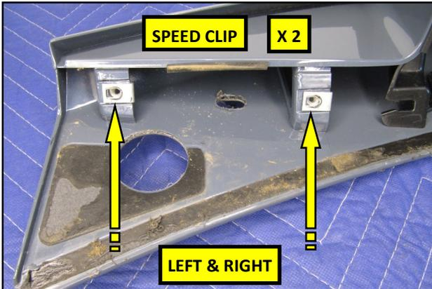
18. Remove the speed clips at each end of the decklid and set them aside.
