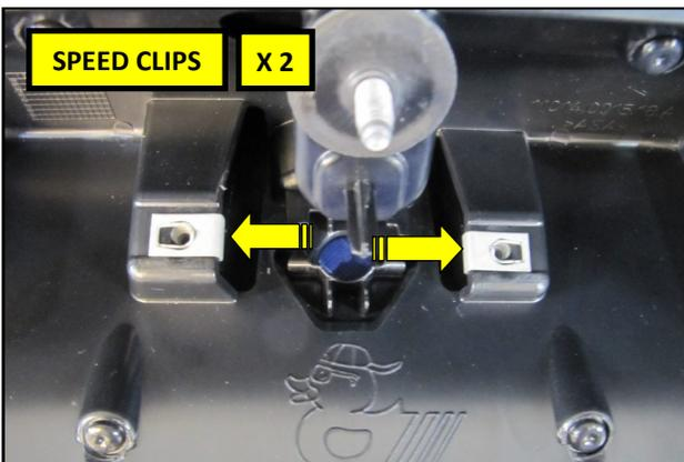
20. Install two supplied speed clips from the hardware pack, onto the center of the RTR Spoiler.
