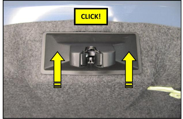
**35.** Reinstall the trunk latch cover from step 2.
