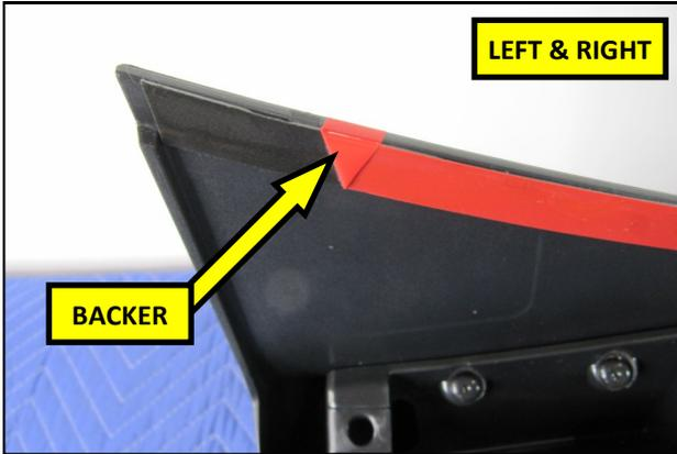
28. Peel back approximately 1 1/2 inch of the tape backer on both ends of the RTR Spoiler and fold it over as shown.
