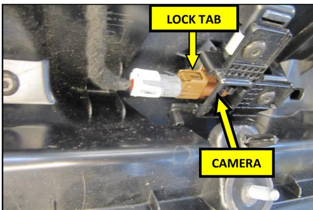
14. Depress the lock tab on the camera connector and disconnect the harness from the camera.
