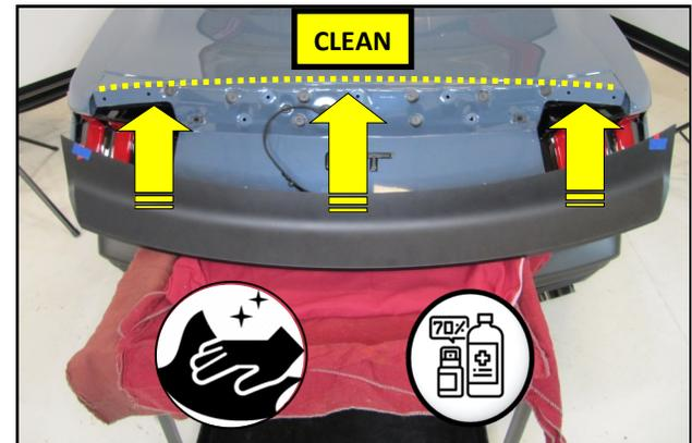
31. Clean the trunk lid, one last time, using isopropyl alcohol. Align the T bolts with the holes in the trunk lid and slide the RTR Spoiler onto the vehicle.
