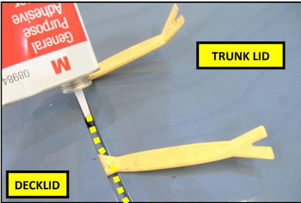
11. Saturate the adhesive at the leading edge of the decklid with adhesive cleaner. When the adhesive has fully softened, carefully pry the deck lid off of the trunk lid using plastic trim tools.
