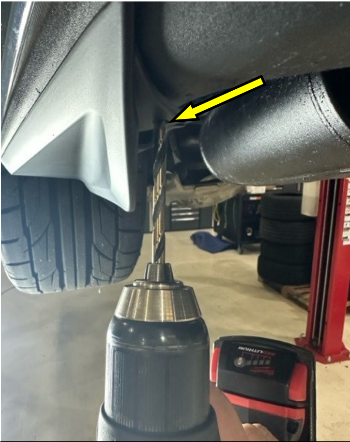
6. Using the quarter splitter as a guide, drill a ¼" (6mm) hole for the final fastener location. Clean up loose plastic bits and be sure hole is clear of debris before proceeding.
