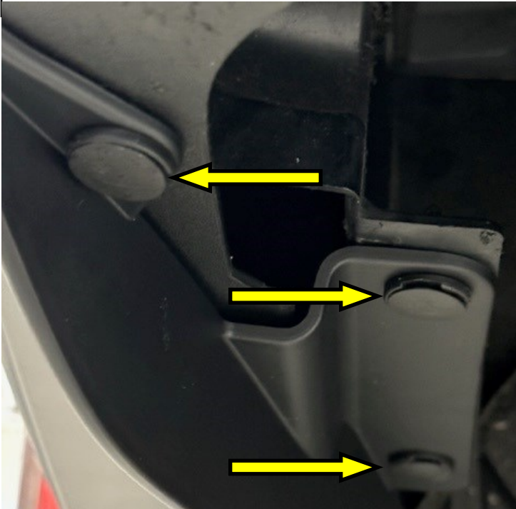
8. Be sure all push pins are flush. Repeat steps on opposite side of vehicle to complete installation.
