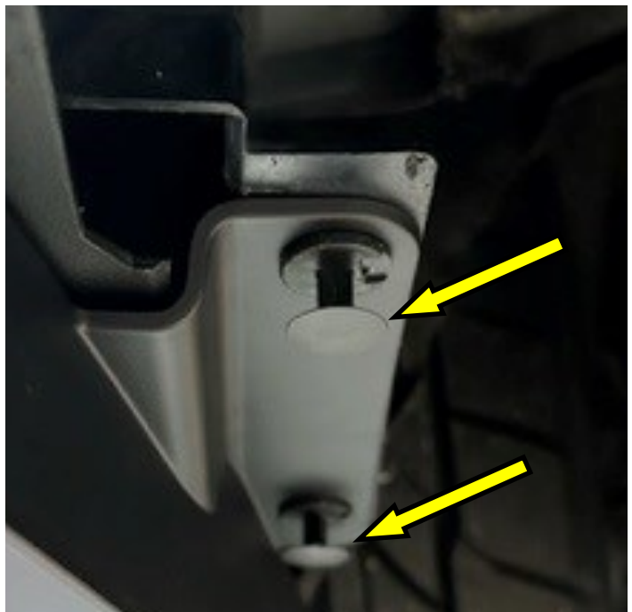
5. Install two push pins as shown. Ensure these go through the quarter splitter as well as the lower bumper cover.
