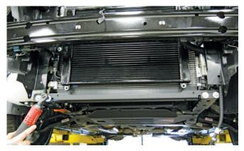
Remove the four (4) bolts holding the LTR to the bumper brackets.
