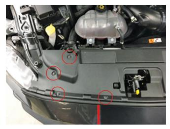
9. Remove the two (2) 7 mm screws and six (6) 8 mm screws from the upper lip of the fascia. Lift the fascia off the alignment pins and forward off the vehicle (this step may require assistance from another person).
