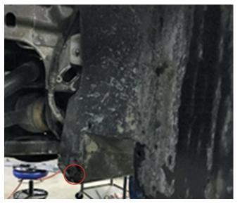
4. Remove the two (2) 8 mm screws from the stone deflector (non-performance package) located on the undertray just in front of each tire. Note stone deflector is not shown but fastener locations are indicated. Repeat on the other side of the vehicle.
