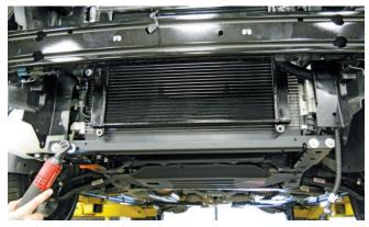
Install two (2) lower LTR brackets (1318-8K224) found in the new kit. Secure each tab to the LTR using two (2) of the takeoff bolt. Torque to 25 Nm.
