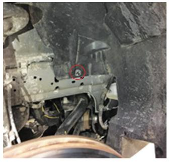
3. Remove the five (5) push pins and remove the fender liner as shown. Repeat on the other side of the vehicle.
