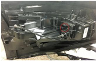
7. Remove the two (2) nuts and one (1) push pin holding the fascia to the fender. Repeat on the other side of the vehicle.
