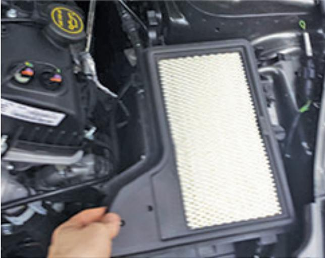
7. Remove the bolt holding the air box to the inner fender using the 10 mm socket.
