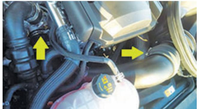
10. Remove the air temperature sensor from the factory air box by twisting counterclockwise and reinstall into the ROUSH filter tube (131523-12B579) by twisting clockwise.
