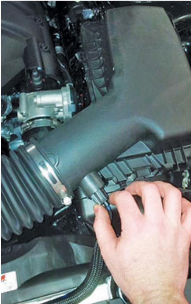
4. Loosen the clamp at the air box from the intake tube.
