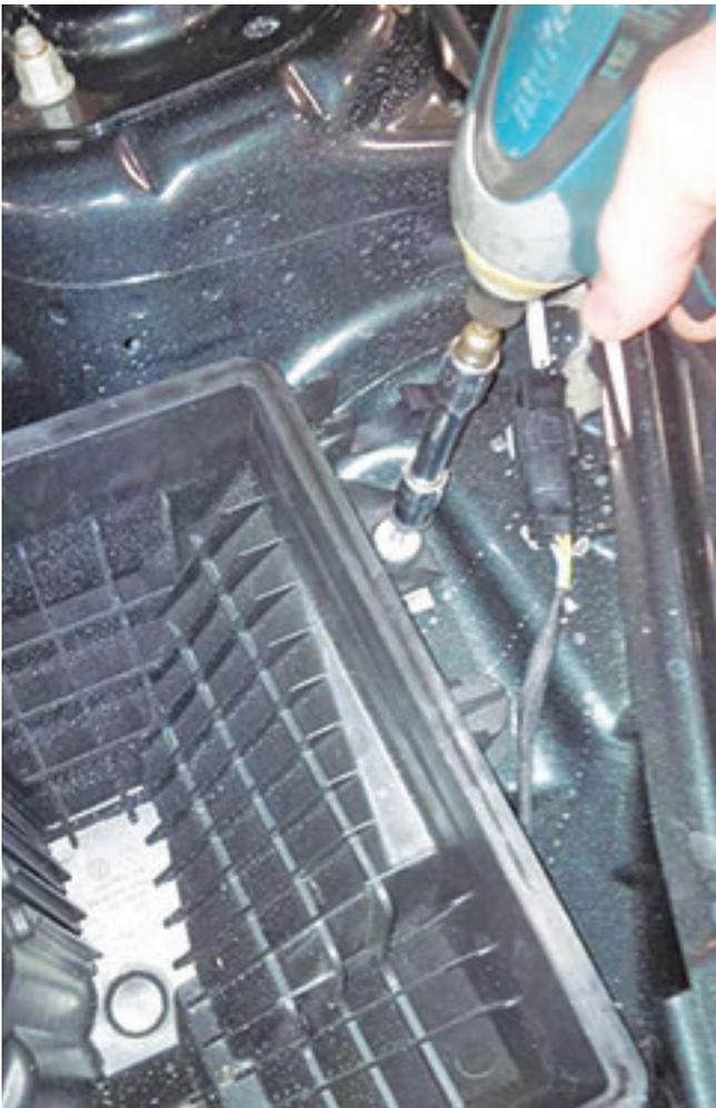
8. Remove the air box tray and dirty air inlet from the vehicle.
