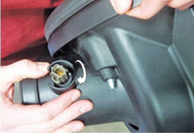
11. Connect the temperature sensor connector.
