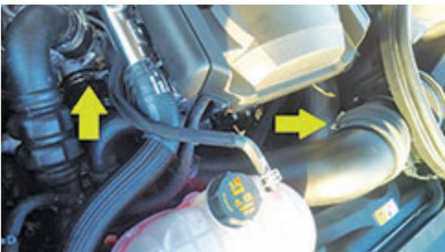
13. Install the PCV tube with the quick connect, making sure it is fully seated. Install the recirculation valve hose with the constant tension clamp.
