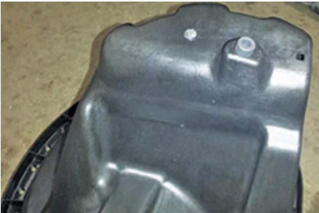
4. Insert the dirty air inlet (1315-9F763-A) into the air box (131550-9A612).
