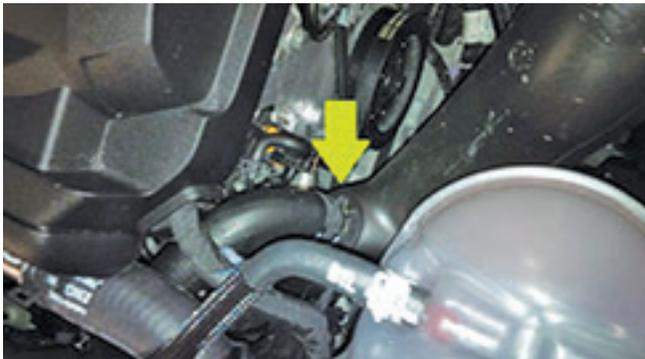
11. Remove the PCV quick connect fitting from the stock clean air tube.
