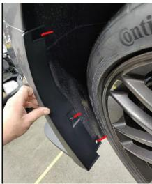
2. Measure on the TOP of the canard as shown, and make a cut line.
