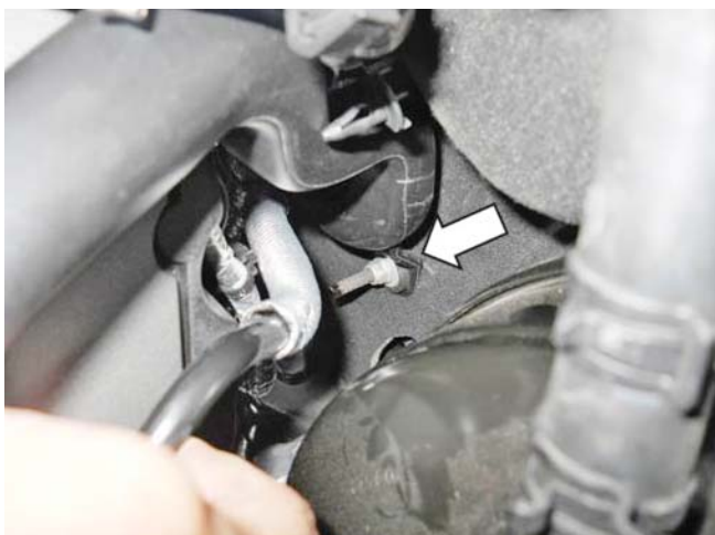
13. Using a 10 mm wrench or deep-well socket, remove the nut retaining the induction resonance tube to the firewall behind the driver side cylinder head.
