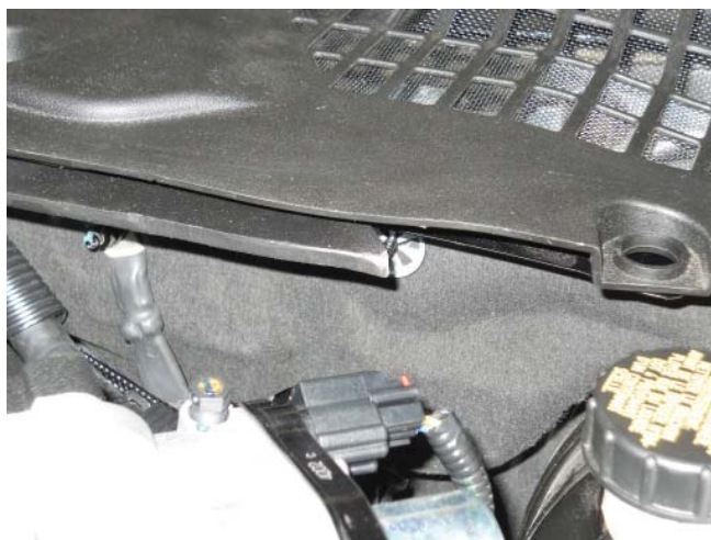
Exposed point on modified K-brace, shown installed
