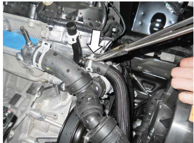
Degas hose from bottom of bottle
