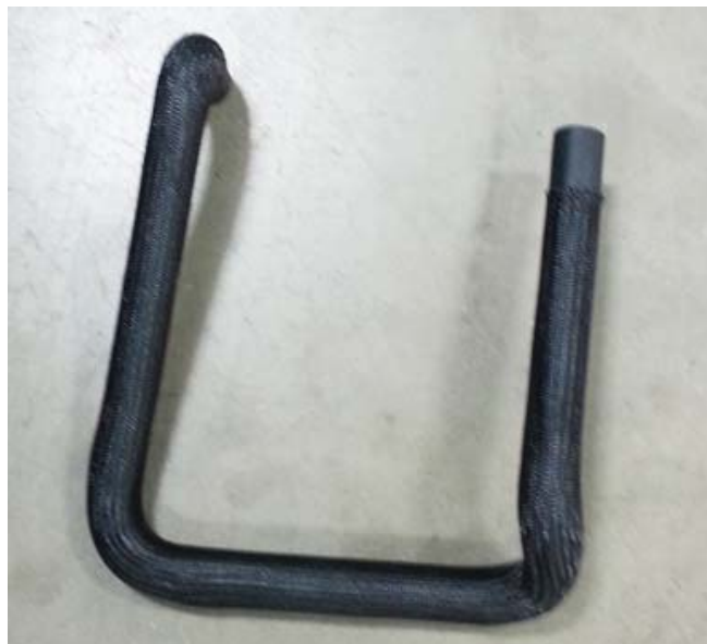
Intercooler pump outlet hose (1315-6K236)
