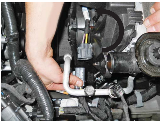
Fan shroud electrical connector
