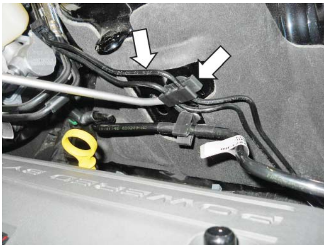
Remove tube from retainer
