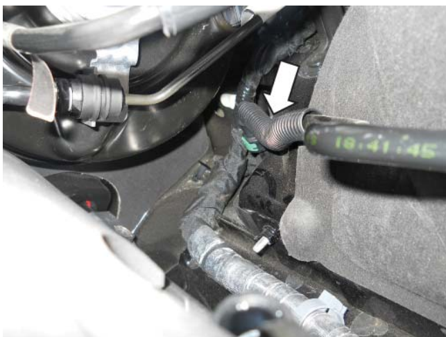
Disconnect green quick connect fitting
