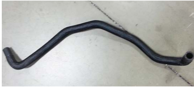
Intercooler pump inlet hose (1315-8D029)
