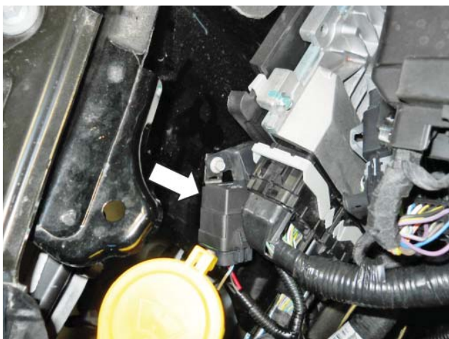
Relay bolt, front side
