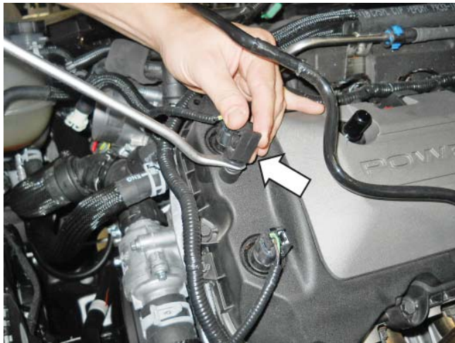
Remove retainer on cam cover
