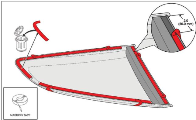
4. Install the window scoop onto the rear quarter glass using the edge of the window's rubber surround molding as a guide. Do not allow the exposed double-sided tape to adhere until the window scoop is properly aligned, then press down.
