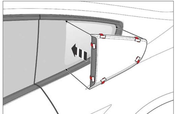
5. Remove all the tape liners in the order shown below. Be sure to remove the tape liners in the direction indicated.
