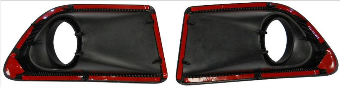
4. Peel the backing on the two-sided tape and install the fog lamp bezels onto the bumper cover.
