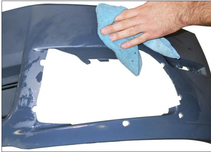
2. Using the 3M adhesion promoter 4298 (021200-27571) found in hardware kit (1313-FGBZHWK), wipe the outer rear edges of the fog lamp bezels.
