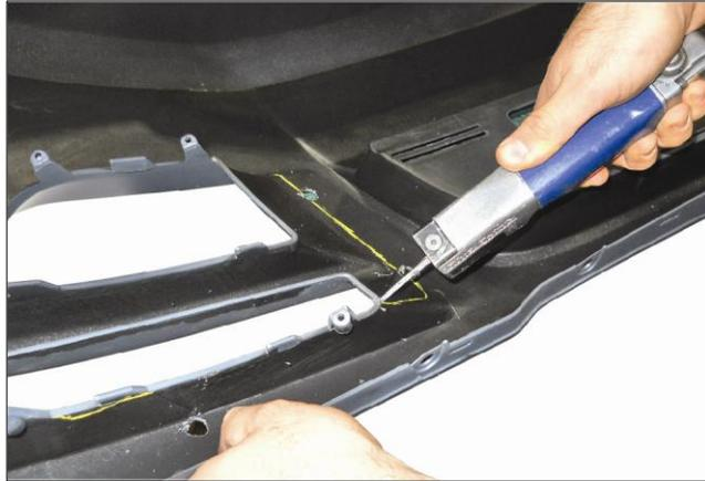
8. Deburr the cut edges on the bumper cover and repeat steps 2 through 8 for the opposite side. Once both sides of the bumper cover have been cut, test fit the fog lamp bezels for proper installation.
