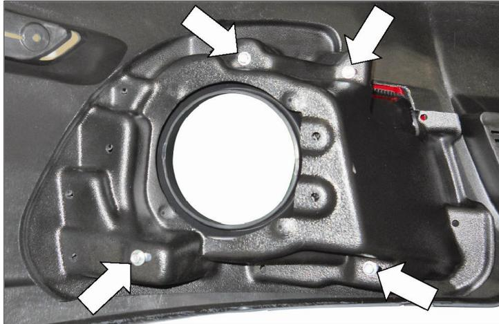
6. Install the seven (7) outer screws (24A000009-G18Q) found in hardware kit (1313-FGBZKIT) on the LH and RH fog lamp brackets (1313-17267 and 1313-17268).
