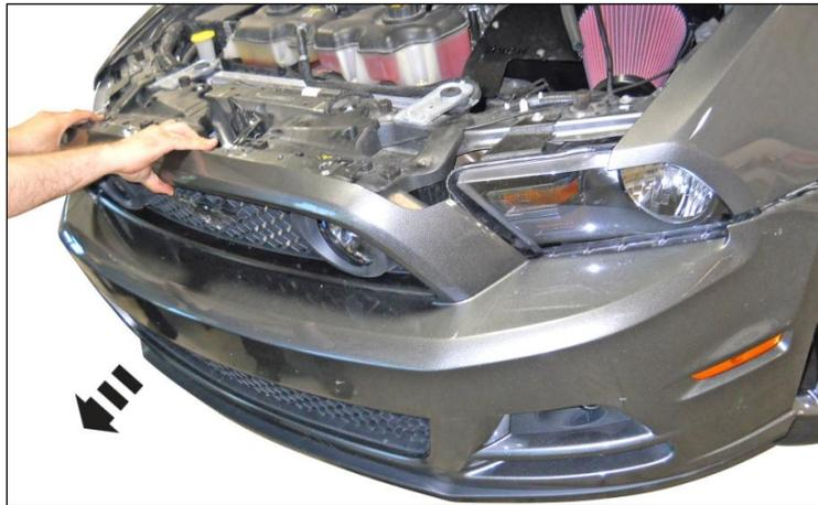
9. Release the five (5) retaining tabs and remove the fog lamp delete panel from the bumper cover.
