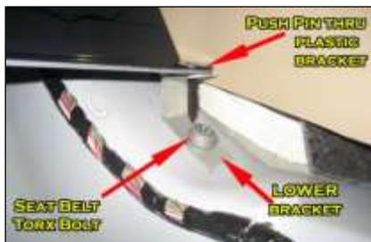
5. ← Use the supplied plastic push pins to connect the lower lip to the Lower brackets. Tighten lower bracket Torx bolts.
