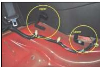
2. Install the 2 **larger plastic brackets** where the previous seat backs mounted. Use the factory black M8 x 1.25 bolts that were removed from the car in earlier steps.
