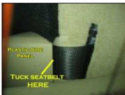
7. ← Tuck the disconnected seatbelt straps behind the side panels, out of view. Do this by removing the 2 push pins on each side of the panel which allows you to pull the plastic back far enough to tuck the seatbelts into.
