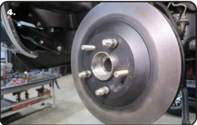
**4.** Install the rotor on the hub. Thread some lug nuts on the threads of the hub to hold the rotor tight on the hub.
