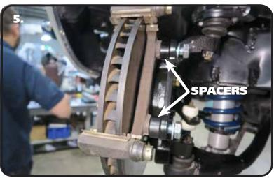
**5.** The kit includes spacers that will be installed between the caliper bracket and caliper mount. Install a M12 flat washer on each of (2) M12-1.75 x 50mm hex bolts. Insert the bolts through the caliper bracket, installing a spacer on each bolt. Line the caliper mount up with the hardware and thread in the bolts.
