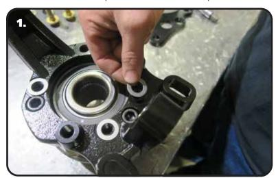
**1.** Lay a .062" thick, 1/2" ID shim on each of the caliper brackets (3) mounting holes.
