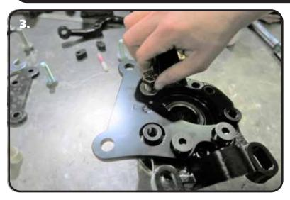
**3.** Insert a  $1/2"-13 \times 1 \cdot 1/4"$  flat head socket cap screw in each of the lower mounting holes. Install a 1/2" flat washer on a  $1/2"-13 \times 1 \cdot 1/4"$  hex bolt and insert it in the upper mounting hole. Tighten the hardware to 75 ft-lbs.
