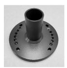
6 speed bearing kits include a collar that mounts to the front plate of the transmission. This plate is designed so that it can be mounted in several positions in order to align the bearing ports to point to the opening in your bellhousing.
