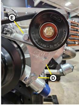
Due to the numerous aftermarket pulley manufacturers and the vast number of different pulley sizes available, you must measure and verify the belt length that is needed for your specific application.
