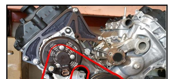
8. Install (3) 8MM flange nuts to secure the alternator bracket to the engine.
