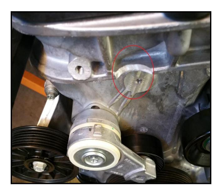
3. Remove the 3 timing cover bolts as illustrated below.
