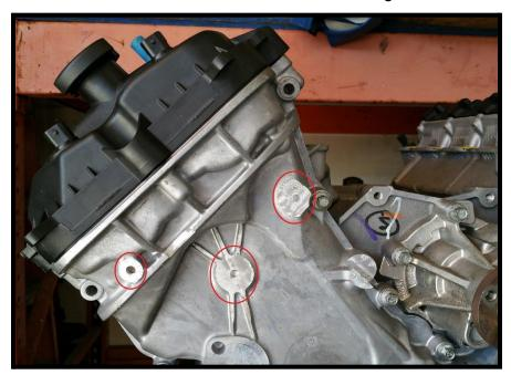
2. Cut a relief into the horizontal rib of the timing cover as illustrated below. The center of the cut should be 1/4" deep.
