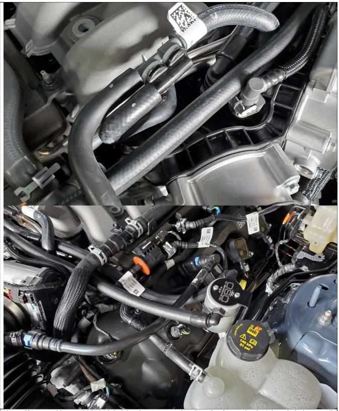
Mount J&L assembly to vehicle with bolt/stud you removed earlier. Don't completely tighten bolt down until you reinstall the engine cover. Check hoses for final fitment and tighten bolt.
