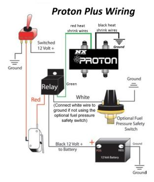
NOTE 1: The wires in the red heat shrink tubing go to positive (+12v), green wire on the relay, and the wires in the black heat shrink tubing go to negative (ground).
