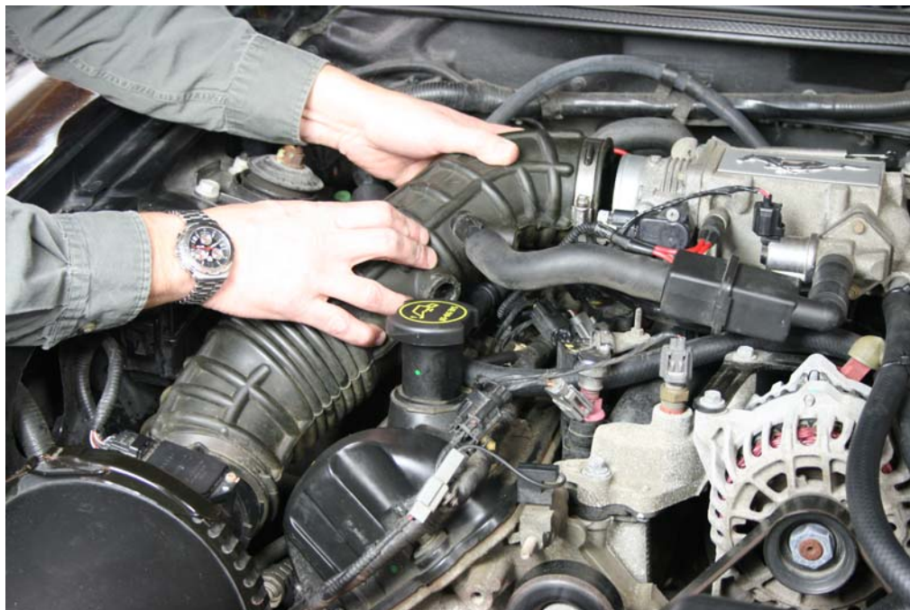
Step 27: Re-Install Air Intake hose to Throttle Body
