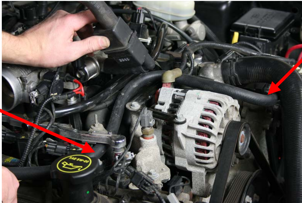
Step 16: Route 1/2" hose from Air Oil Separator to Valve Cover as shown
