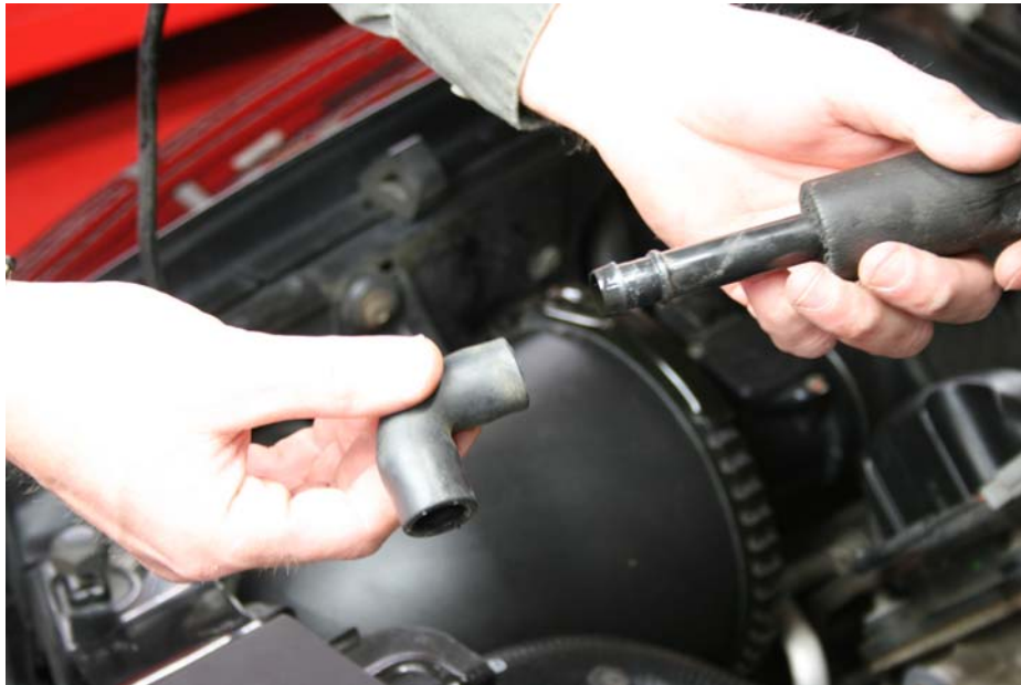
Step 17: Remove 90 degree fitting from PCV tube previously removed
