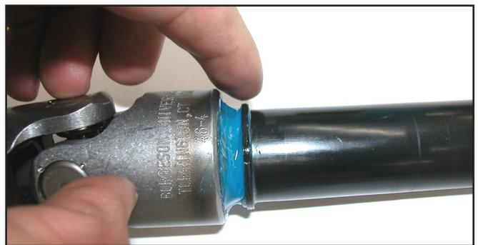
12. Allow the steering shaft to sit for an hour to ensure that the silicone is dry before continuing with the rest of the installation.
