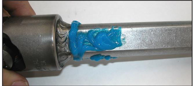
10. Slowly slide the plastic sleeve removed in Step 5 over the upper half of the MM Solid Steering Shaft, until the flanged portion of the sleeve is touching the weld bead.
