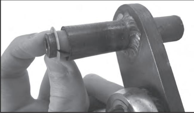
31. Mount the pedal arm in the upper pair of holes, re-using the OEM pivot bolt & nut.
