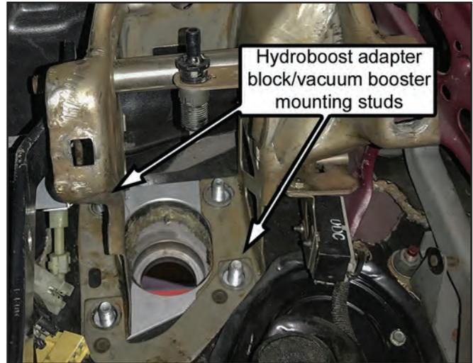
13. Remove the master cylinder and brake booster from the car. Take care not to spill any leftover brake fluid.
