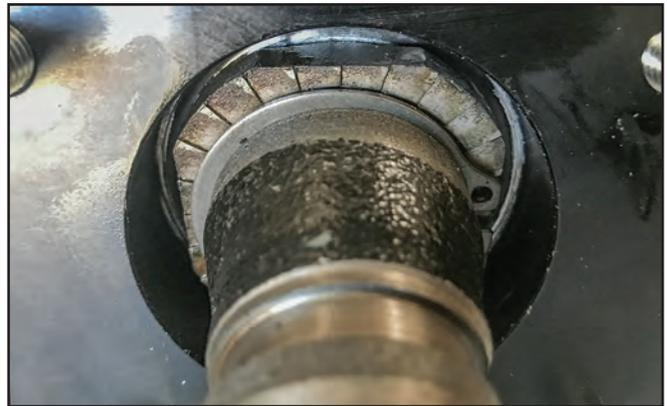
40. Reinstall circlip.
