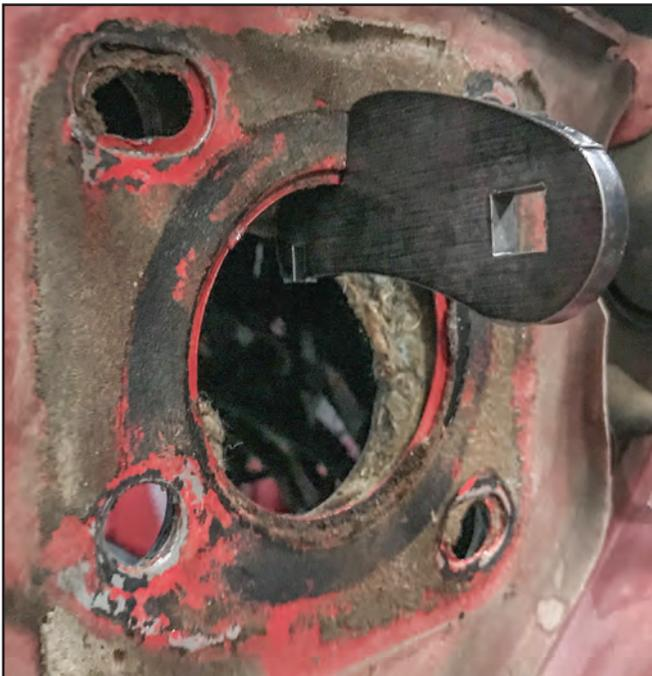
28. With the supplied bending tool, slowly bend the upper portion of the firewall inwards towards the interior of the car. Slowly work the metal between the 10 o'clock and 2 o'clock positions a small amount at a time.
