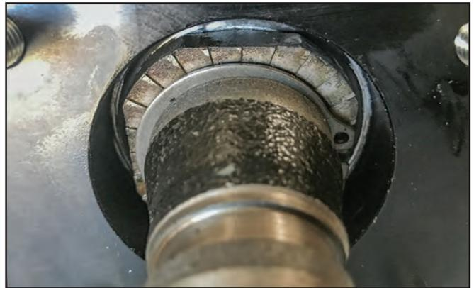
40. Reinstall circlip.
