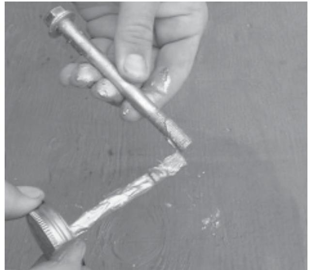
5. Slide *three* 7/16" Grade 8 washers onto the bolt. Slide the 7/16" bolt through the hole of the Bushing Removal Cup (the larger of the two cups). Place the bolt and the cup over the flanged end of the control arm bushing in the differential.
