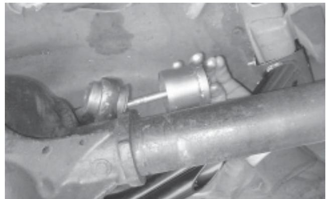
6. Place the 1-3/4" diameter x 3/8" thick disc onto the exposed end of the bolt.
