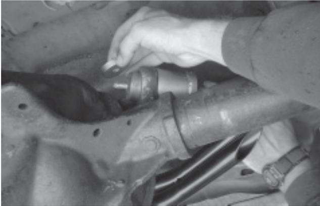
7. Place *three* 7/16" Grade 8 washers over the exposed end of the bolt and thread the 7/16"-20 Grade 8 Hexnut onto the bolt.
