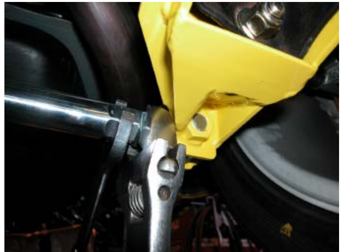
Incorrect- The rod ends are not aligned
