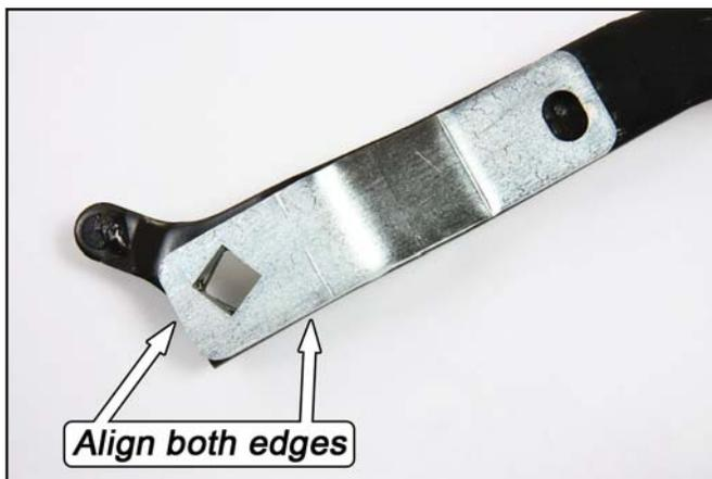
5. Once the edges are aligned, tape the MM Clutch Pedal Adjuster to the OEM clutch pedal lever as shown. This will ensure that the alignment of the part doesn't change while locating the transfer punch in the next step.
