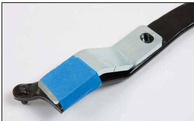
6. Mark the location for a hole flush with the left-hand side of the adjustment slot of the MM Clutch Pedal Adjuster as shown in the picture below. The preferred method is using a 13/32" transfer punch against the edge of the adjustment slot. Once marked, remove the tape applied in Step 5.
