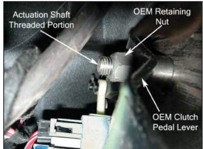
3. Remove the retaining clip from the clutch lock-out switch shaft. Remove the OEM clutch pedal lever from the square-shaped shoulder on the actuation shaft. Rotate the OEM clutch pedal lever to facilitate the removal of the clutch pedal lock-out switch arm. Remove OEM clutch pedal lever from the car.
