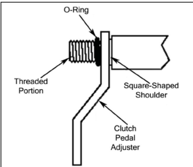
10. Position the OEM clutch pedal lever on the actuation shaft with the square-shaped hole over the O-ring on the threaded portion of the actuation shaft.
