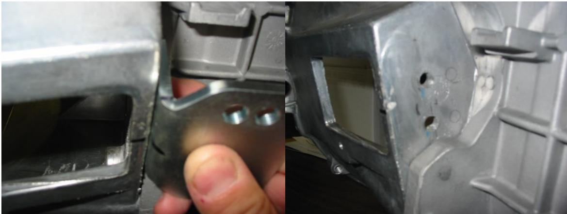
3.3 Install bracket on bell housing with 5/16” bolts and lock washers.
