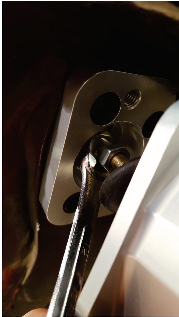
Silver nut used for adjusting 1.4" gap. Gold nut gets tightened once gap is set.
