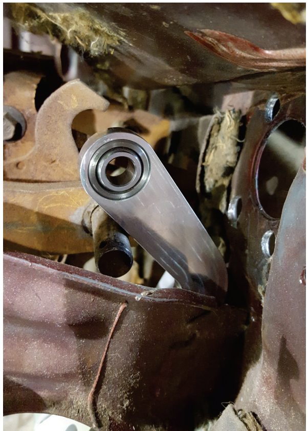
Pre-assembled inner firewall parts and initial position of the push lever shown.
