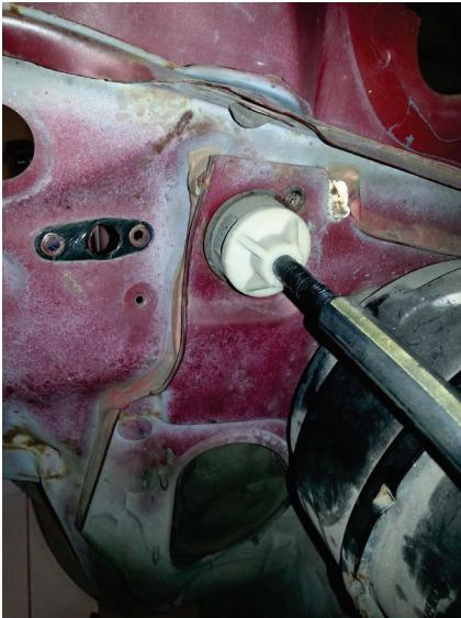
Cable installed, Cable removed, pedal linkage left installed with all necessary parts removed.
