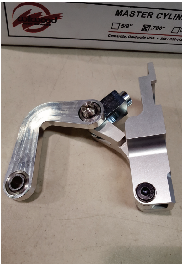
Pre-assembled inner firewall parts and initial position of the push lever shown.
