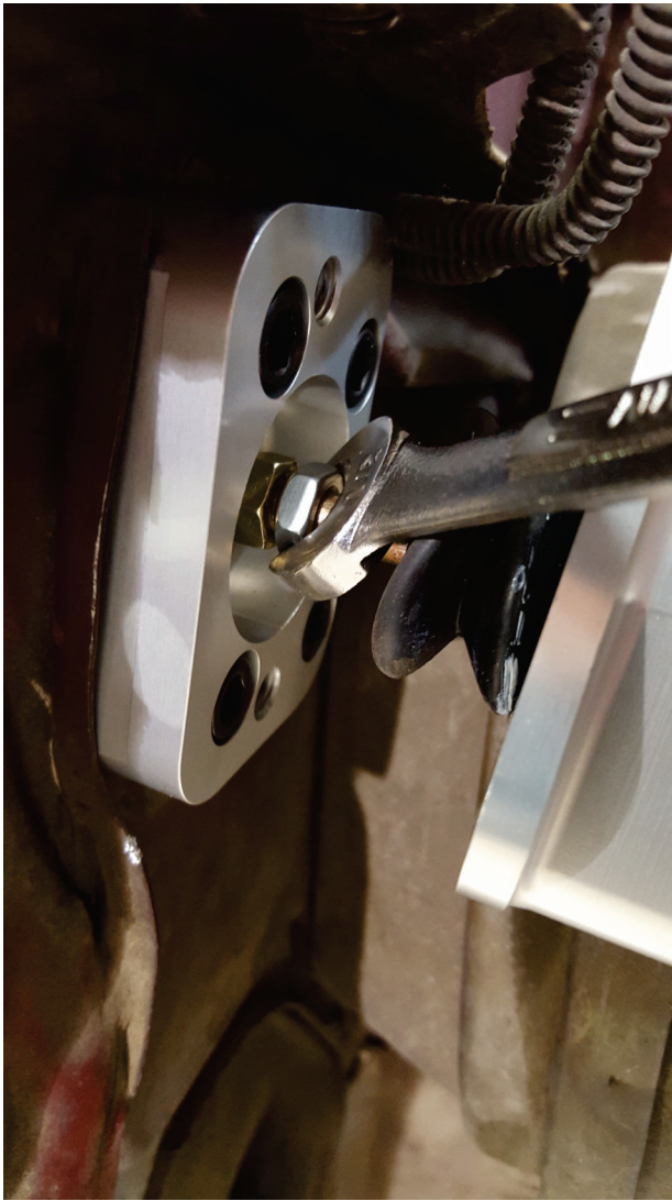
Silver nut used for adjusting 1.4" gap. Gold nut gets tightened once gap is set.
