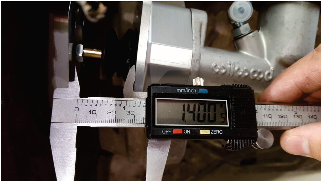
Silver nut used for adjusting 1.4" gap. Gold nut gets tightened once gap is set.
