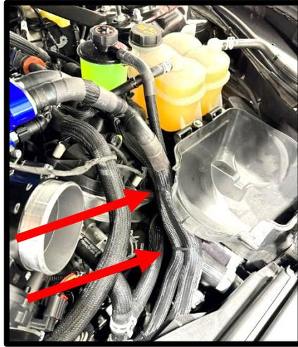
127. Review intercooler circulating pump relay harness diagram below before installing. **\*NOTE:** You're required to remove stock fuse from instructed fuse location, install this into the fuse tap to properly complete the circuit. Failure to do so may result in codes and/or poor performance.
