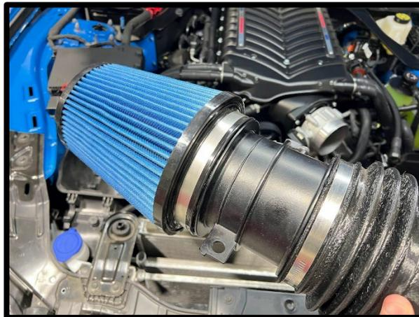
140. Install the MAF housings to the airbox brackets using supplied stock fastener to supplied brackets.
