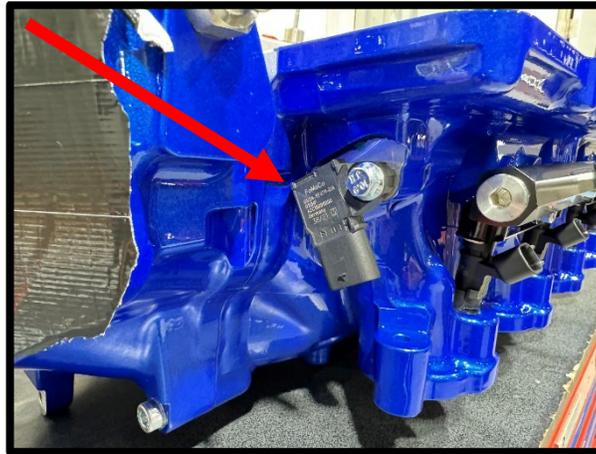
84. Install supplied electronic throttle pigtail to the factory **RH/PASSENGER SIDE** electrical connector. Push until it locks in place, then lock the safety lock. Route to **LH** side of vehicle for later connection to throttle body. **TIP:** When pressing together, hold the wires and connector to ensure the wires cannot come loose during connection.
