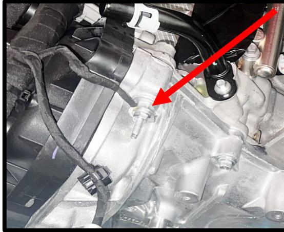
65. Use supplied (4x) 8mm x 90mm in the (3x) lower holes to secure the idler plate to the front of the passenger side of engine, install hand tight. Using a 6mm allen, torque to 22 lbs-ft.
