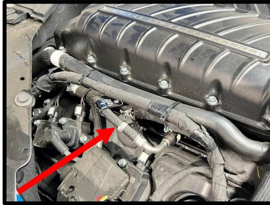
104. Connect factory fuel inlet line to the driver side fuel fitting, press until it clicks and locks in place.
