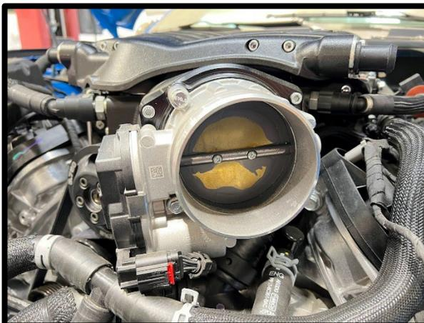
136. Connect previously installed throttle extension pigtail to the throttle body electrical connector. Secure wiring using zip-tie. **NOTE: Failure to secure wire may result in the wire catching the belt system!**
