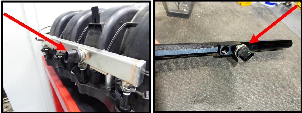
75. Install supplied (2x) #2-906 Viton oring to (2x) 45mm long 9.49mm fuel fittings. Apply light amount of grease to oring for ease of installation and install fitting. Install fittings, one per rail.
