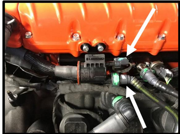
108. Install supplied 3/8" ID x 5 1/2" with 55deg quick connect fitting hose (#5000030) to the EECPV barb fitting and **LH** quick connect fitting on SC inlet. Push until it clicks and locks into place.
