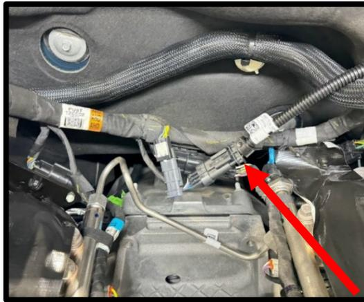
87. Install supplied IMRC electrical connector plugs (2x). Zip-tie to harness.
