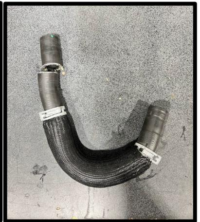
61. **(Auto Transmission)** Connect U shape hose back to stock tees, install/position to **FRONT** side of radiator hose (this stops it from getting to water pump pulley. Rotate the factory hose retainer and connect to this hose to secure in place.
