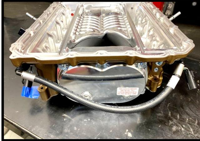
81. Install supplied 1/4" ID bypass actuator to bypass nipple and 1/4" 90deg nipple on SC inlet. **CAUTION:** Do not open/close bypass actuator by hand. This may damage actuator internally. It only moves properly with equal vacuum/boost at the actuator reference port.
