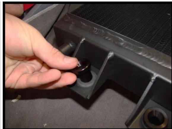
112. Install the supplied (4x) hex coupling nuts to the factory bolt threads on the back side of the front bumper support (2 driver side, 2 passenger side) using a 16mm wrench.
