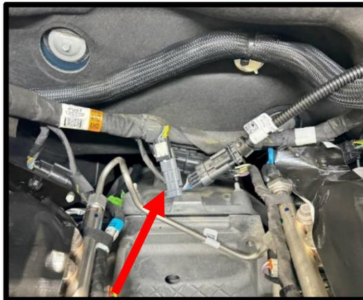
88. Install supplied wiring plug (1x) to the **LH** throttle electrical connector. Zip-tie harness away from belt system.
