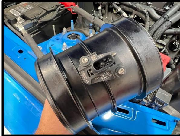
139. Install supplied filters to MAF housing, secure using supplied filter clamp. Install the MAF housings into the Y tube (for ease of installation), pre-install #80 hose clamp to Y tube, leave loose until later.
