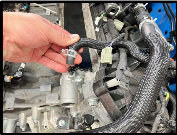
57. **(Auto Transmission)** Release the hose clamp from transmission fluid valve and hose facing down from tee. Remove plastic hose retainer from oil cooler solenoid hose.
