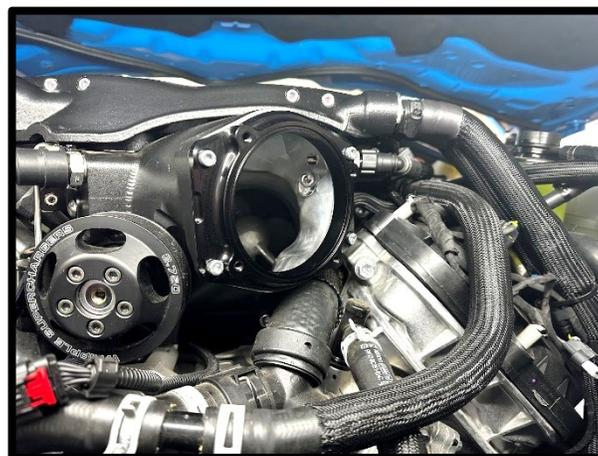
135. Install supplied (1x) #2-045 V75BR oring to TB adapter. Install the stock throttle body using the (4x) 6mm x 35mm HHFCS bolts using a 10mm socket.
