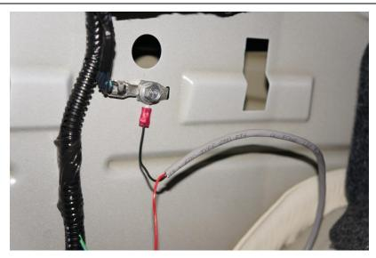
3. Attach the Exhaust Valve Control box Ground Lead under the Body Ground Bolt and tighten.
