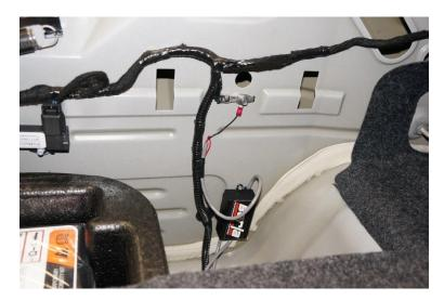
8. Mount the Exhaust Valve Control Box to the rear Panel of the trunk using the included Hook and Loop Fastener. Make sure you mount the box low enough to clear the rear trunk trim panel.
