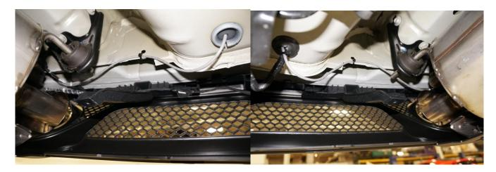
9. Connect the Exhaust Valve Actuators Before Installing the Muffler Packs. Access to the Plugs is very difficult once the Mufflers are installed. Use a wire tie to retain the wire to the rear Panel of the car. There are factory holes for you to use. Be sure to leave a small amount of slack in the harness but, not so much the wiring is visible from behind the Vehicle.
