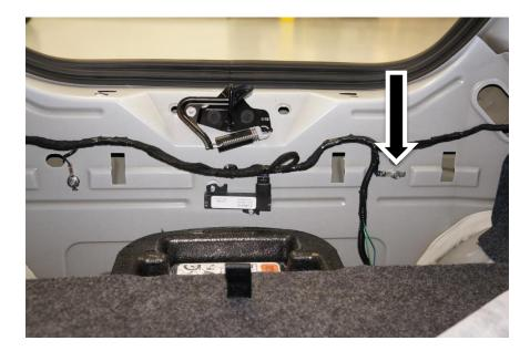
2. Locate the Ground Screw Located on the trunk rear wall. Loosen this Screw but it is not necessary to remove it completely.
