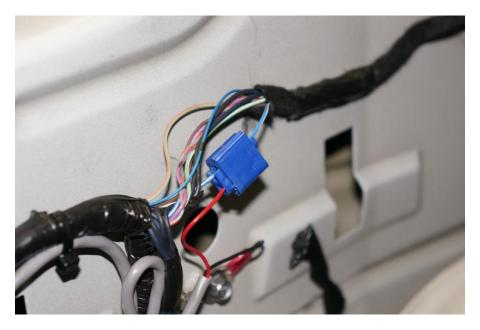
5. Connect the **Red** Power feed from the Exhaust Valve Control Box to the **Blue with a White tracer** using the provided Quick Tap Wire Connector. Re-wrap the harness with Electrical Tape when the connection has been made.
