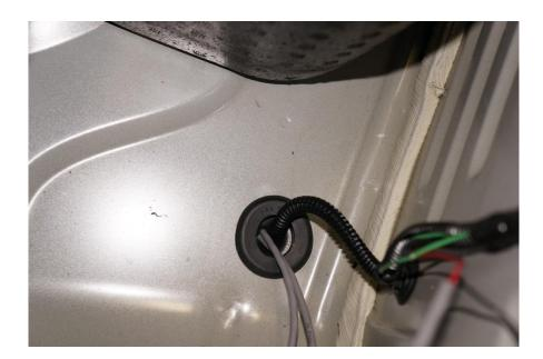
6. Cut a small slit in the Grommet located in the Spare Tire Well on the **Driver** side of the Vehicle and feed the **Short** Exhaust Valve Connector through it.
