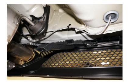
7. Cut a slit in the Grommet located in the Spare Tire Well on the **Passenger** side of the Vehicle and feed the **Long** Exhaust Valve Connector through it.
