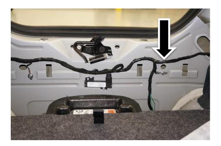
4. Strip off some of the outer loom tape to expose the Wires inside. Locate the **Blue with a White tracer** Wire located in the Rear Tail Lamp Harness that runs across the rear panel of the Trunk. Using a Volt Meter, Ensure that wire has 12 Volts with the key on.
