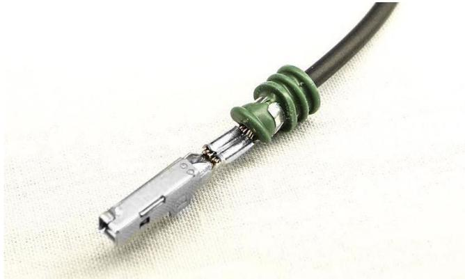
5. When complete, do a pull test. The crimped connection should be as strong as the wire itself. If you're able to pull the crimped terminal off the wire then it wasn't crimped tight enough.
