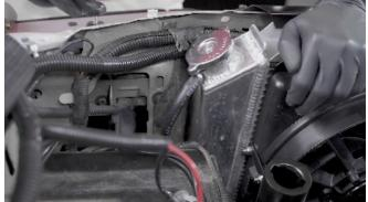
13. Install and wire supplied pig tails to power supply or fan controller of choice.
