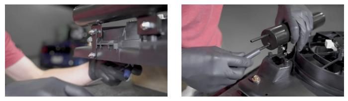
11. Insert lower fan bracket into s-clips, then align & secure upper fan bracket with supplied mounting bolts.
