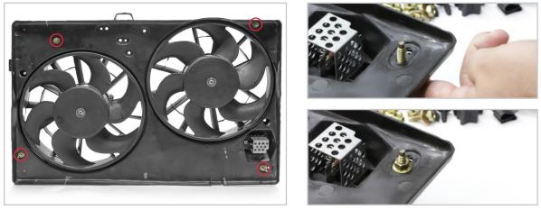
3. Install both brackets with curved edge towards inside of fan assembly. Secure with supplied retaining nuts.
